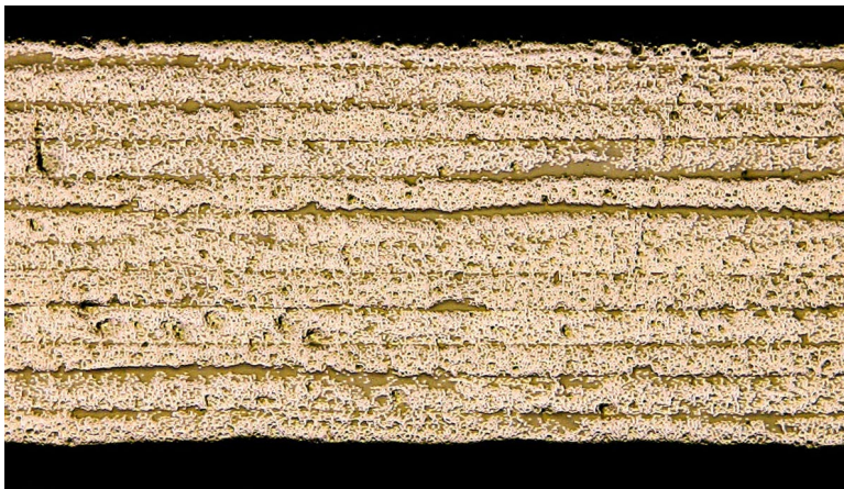
Figure 32(c). Photomicrograph (25x) of edge of [\pm 25]_{3S} aged with load.
