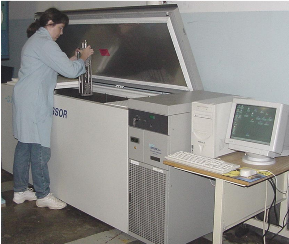
Figure 5. Cryogenic aging chamber.
