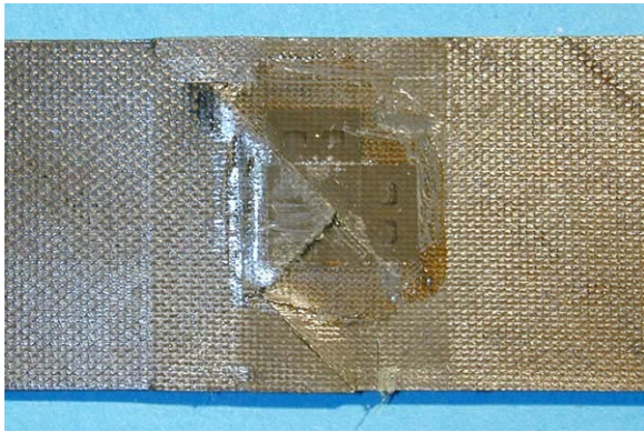
Figure 41(a). Fracture surface of [\pm 45]_{3S} -ply laminate after compression test at room temperature.
