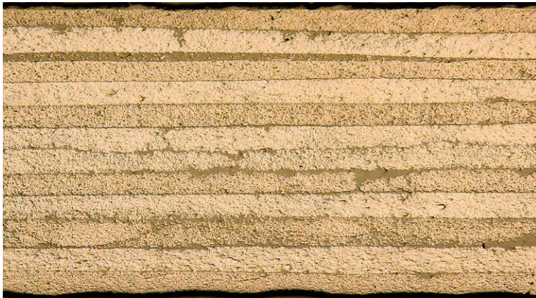
Figure 31(b). Photomicrograph (25x) of edge of [\pm 45]_{3S} aged without load.
