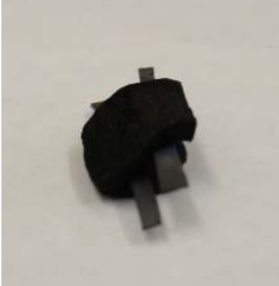
Figure 2-2: Charred ARI-2718 Specimen Showing Warping from Foil Surface
