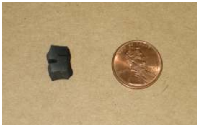
Figure 2-5: Warped Specimen of Charred ARI-2719
