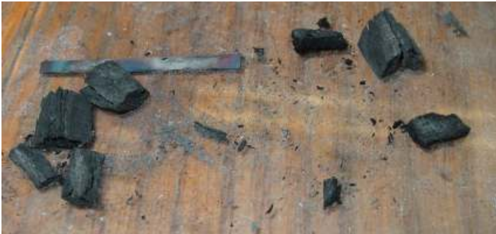
Figure 2-1: Charred ARI-2718 Specimens from Initial Char Procedure
