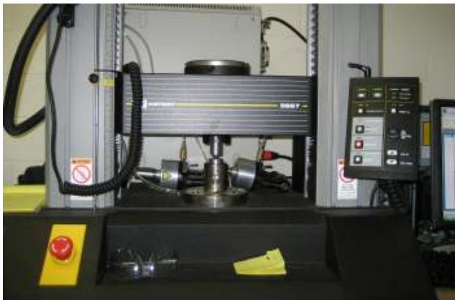
Figure 2-31: Instron 5867 Test Fixture
