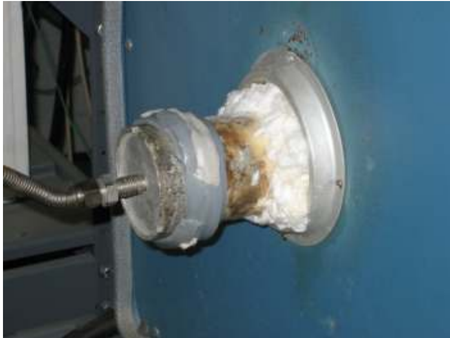
Figure 2-3: Sealed End of Alumina Tube
