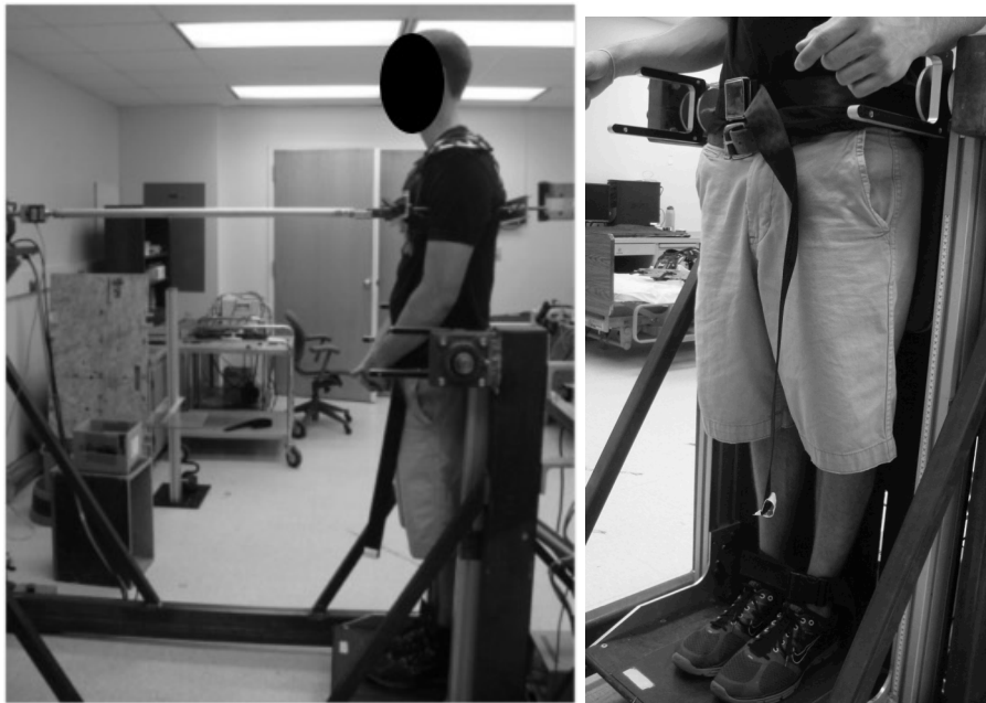
Fig 8(a): Pulling on the rod gives the extensor strength and pushing on the rod gives the flexor strength Fig 8(b): Straps to fix the lower to the back support (Photo taken by the author)
