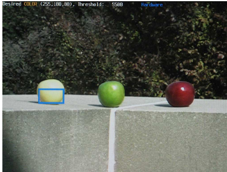
Figure 6.6: The hardware algorithm, attuned to yellow.
