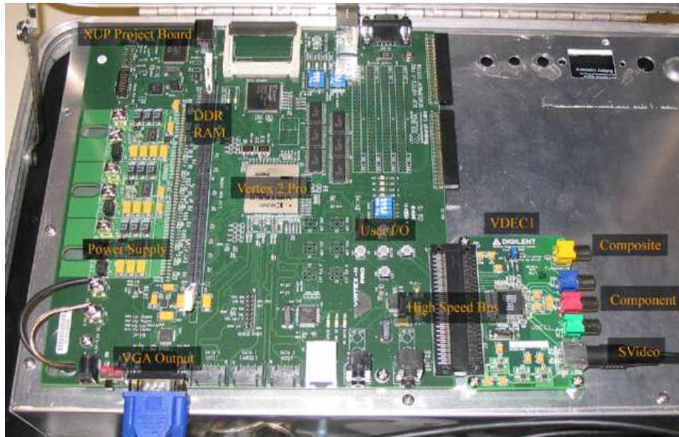
Figure 6.1: The XUP platform with attached VDEC1 video decoder.
