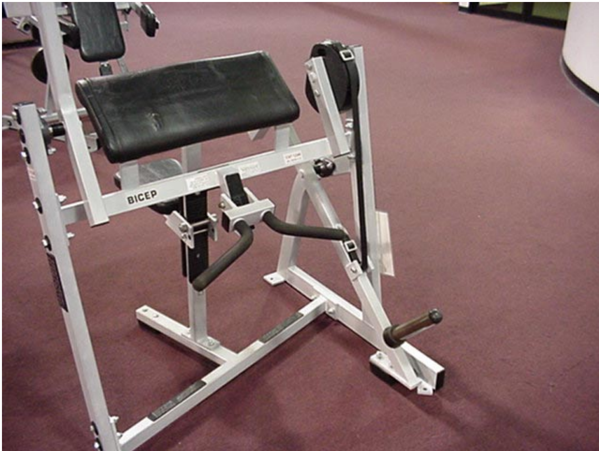
Figure 1-3 Hammer Strength™ bicep-curl machine; uses independent weights.
