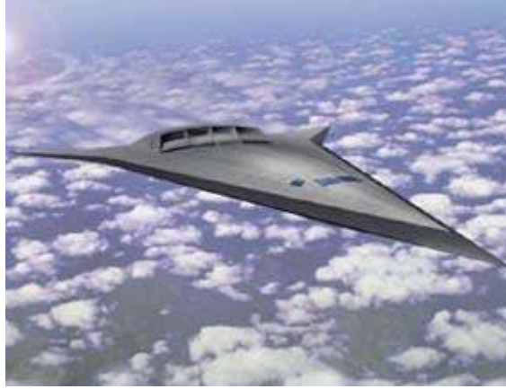
Figure 4. Northrop Grumman Supersonic Tailless Air Vehicle (STAV) configuration 5 .
