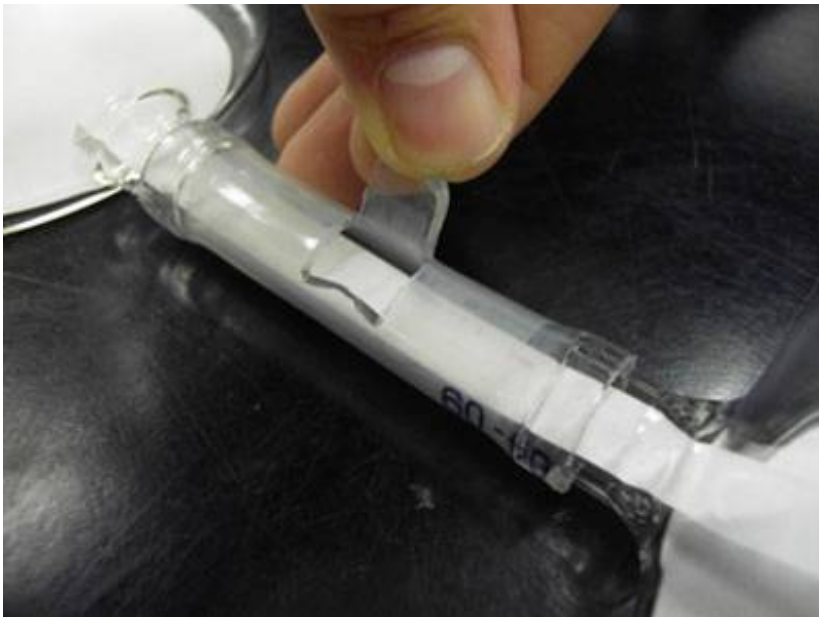
Figure 4-1. Dual choice chamber olfactometer used to determine an individual bed bug's response to a potential aggregation attractant.
