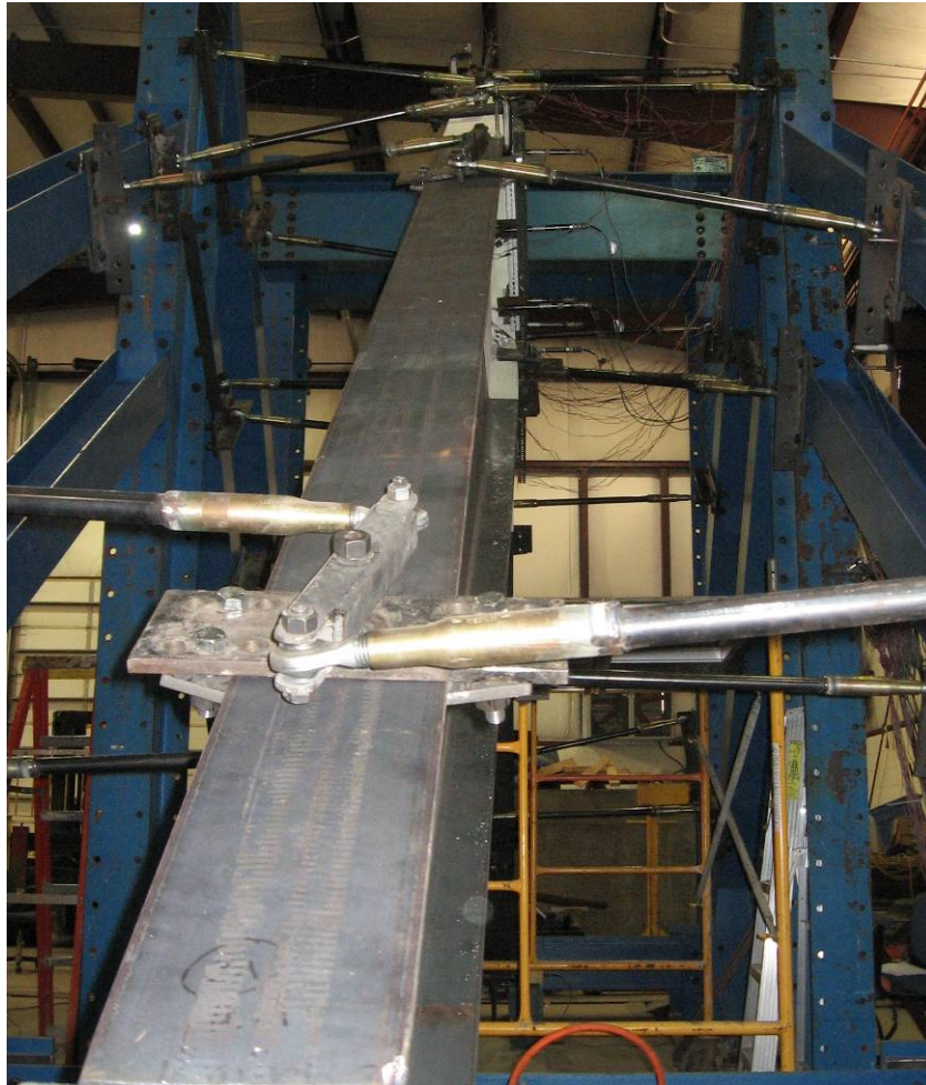
Figure G-1 MH-1-2 Rafter Lateral Torsional Buckling
