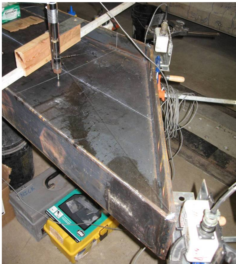
Figure 2-7 SH-1 and SH-2 Web Plane Measurement
