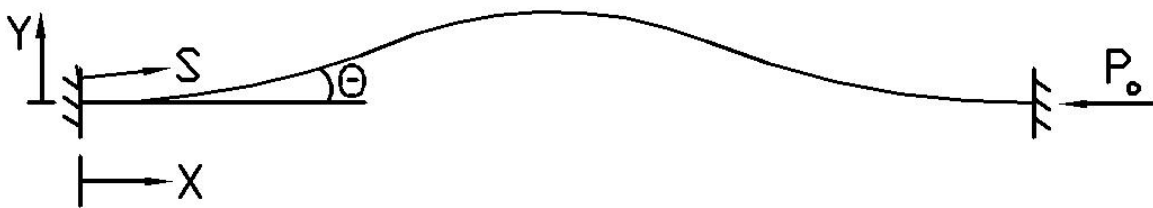
Figure 2.3 Single Buckled Strut Under Static Load P_0
