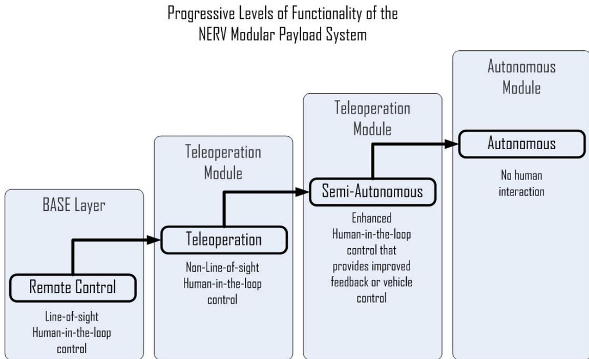
**Figure 50:** Progressive functionality afforded by the modular design of the NERV
