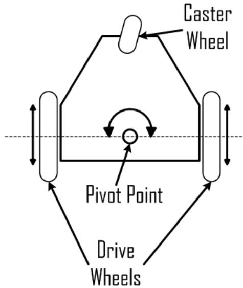
**Figure 27:** Three-wheeled differentially driven mobility platform
