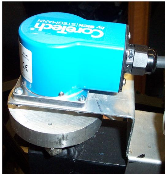
**Figure 72:** Integration of the absolute encoder on the joint
