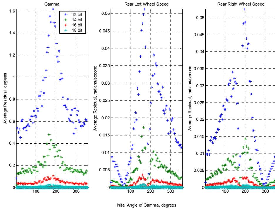
**Figure 99:** Absolute value of the residuals for the first wheel velocity case.
