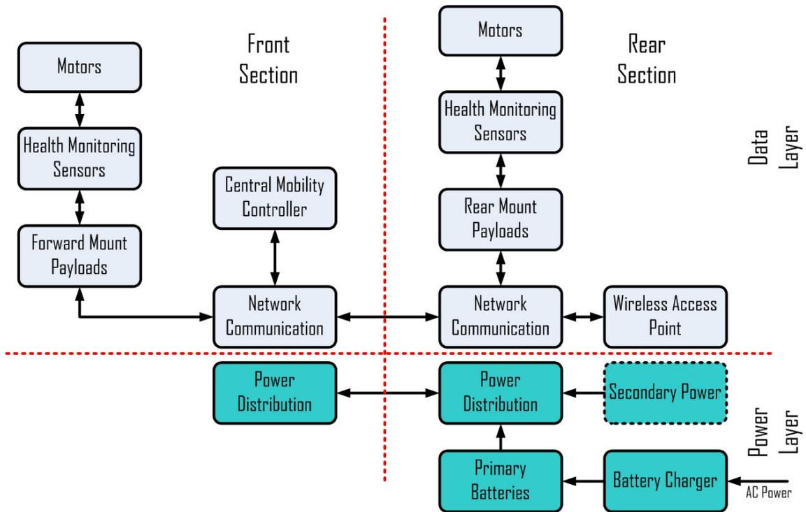
**Figure 63:** System architecture of NERV concept
