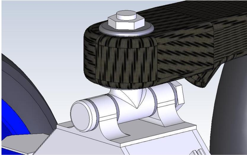
**Figure 61:** Two degree-of-freedom joint assembly
