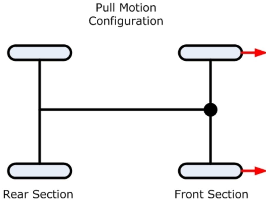
**Figure 105:** "Pull" configuration of the two-body vehicle design
