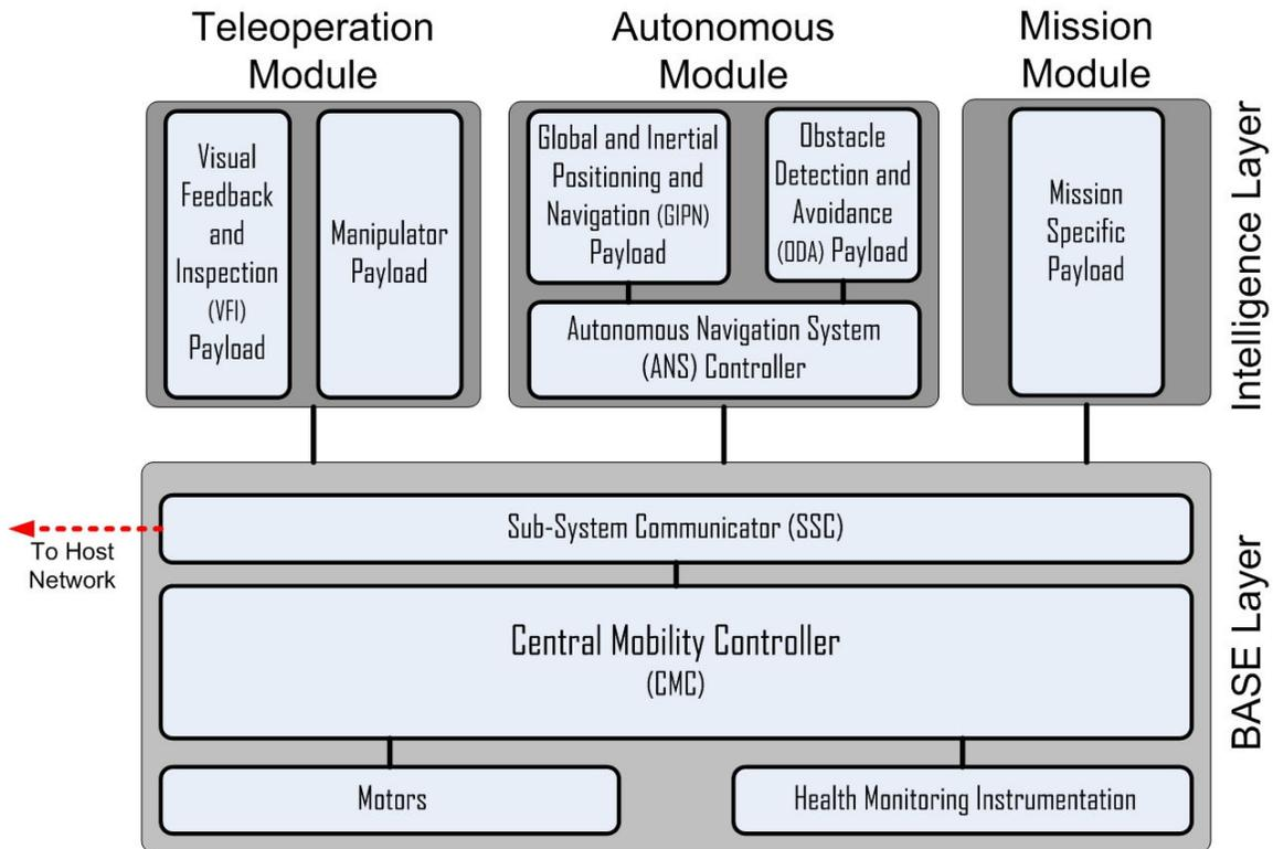
**Figure 49:** Modular payload system architecture
