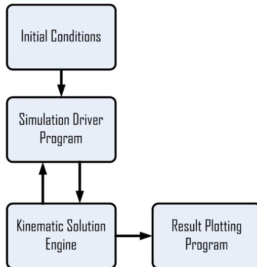
**Figure 38:** Kinematic simulation program architecture
