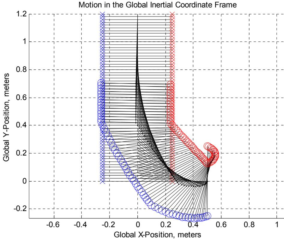
**Figure 98:** Discontinuous motion as a result of an 8 bit encoder to measure body angle
