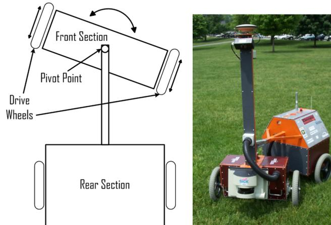
**Figure 22:** Detail of the steering method of Gemini
