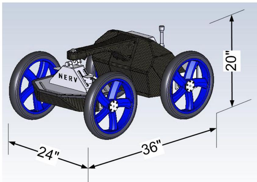
**Figure 57:** Dimensions of the NERV platform
