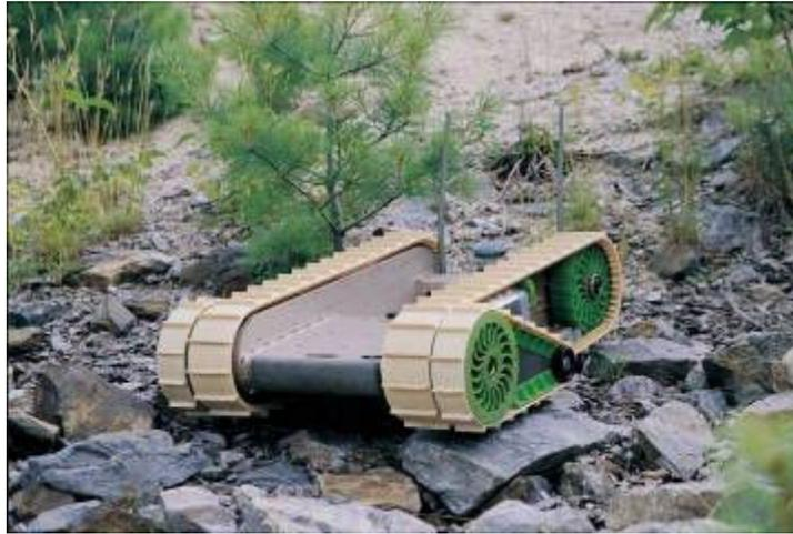
**Figure 29:** iRobot's PackBot utilizes a track system [61]
