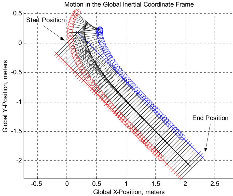
**Figure 44:** Motion of the two-bodied platform with the rear wheels moving to match the velocity of the front wheels.
