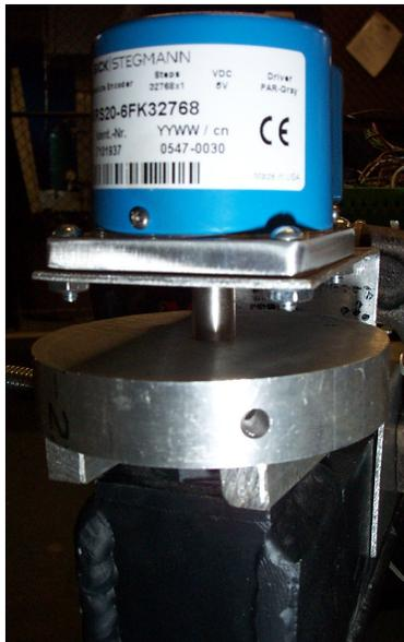
**Figure 73:** Side view of absolute encoder mount
