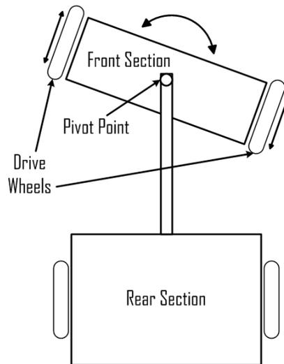
**Figure 28:** Four-wheeled differentially driven mobility platform
