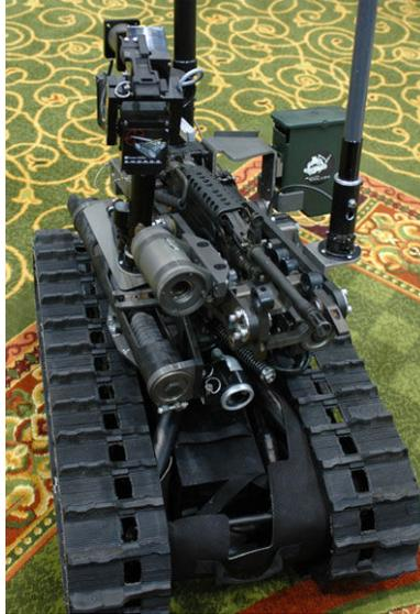
**Figure 17:** SWORDS Talon platform with mounted weapon [40]
