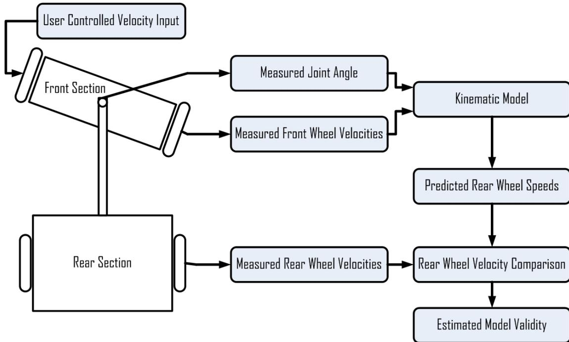
**Figure 70:** Experimental diagram for kinematic model validation
