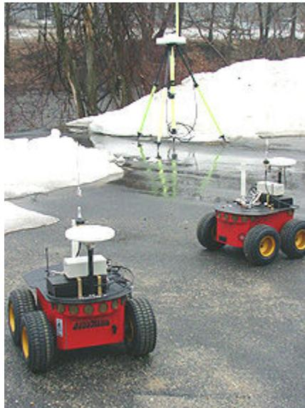
**Figure 30:** Small mobile research robots that use skid-steer wheels [63]
