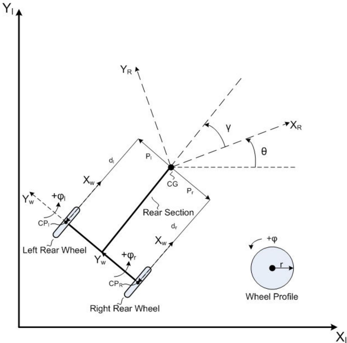
**Figure 37:** Kinematic model of the rear section of the two-bodied vehicle
