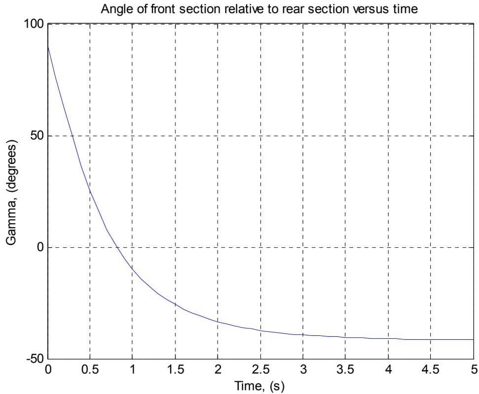
**Figure 42:** Angle between front and rear sections of the vehicle as a function of time for the case presented in Figure 41.
