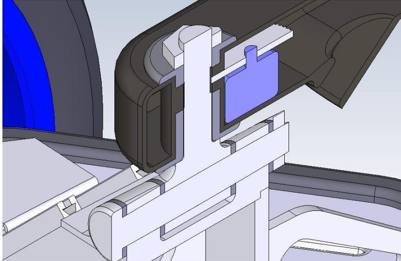
**Figure 62:** Section view of the two degree-of-freedom joint
