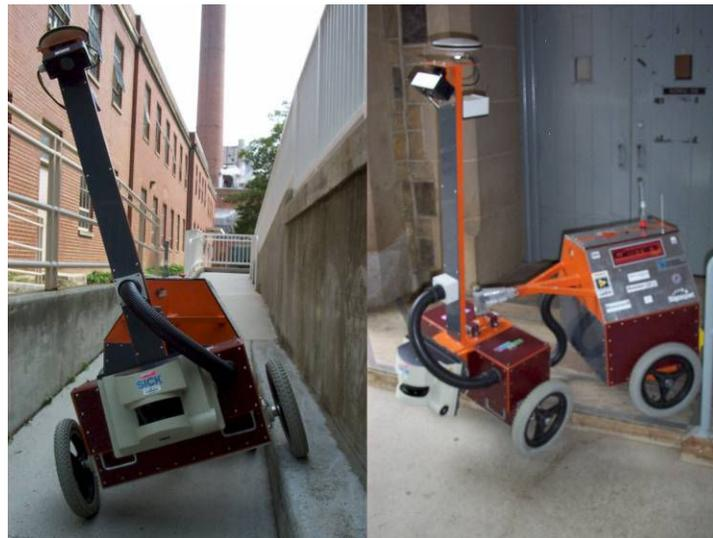
**Figure 23:** The unique mobility provided by the two degree-of-freedom articulated platform
