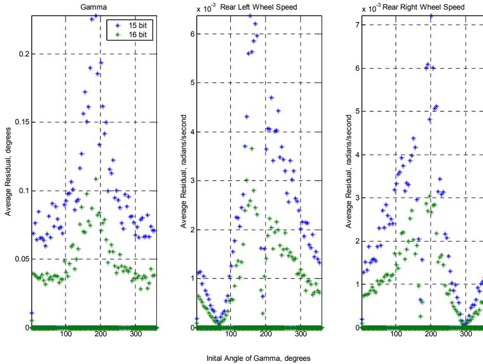
**Figure 106:** Absolute value of the residuals for the instrumented simulation for a 15 and 16 bit encoder.
