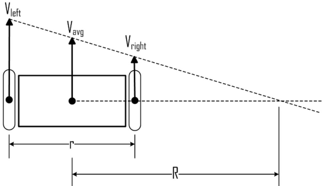
**Figure 31:** Schematic representation of coaxially oriented differentially driven wheels with  $R$  being the vehicle turning radius
