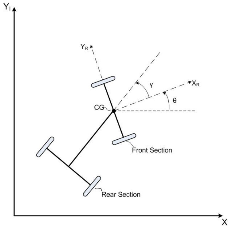
**Figure 34:** Kinematic representation of the two-body articulated mobile robotic platform.
