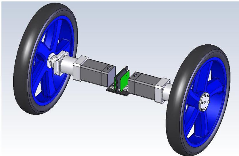
**Figure 60:** NERV drivetrain assembly
