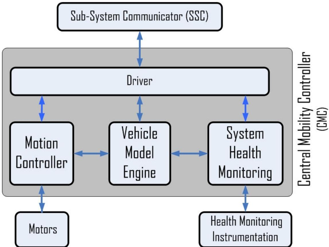
**Figure 51:** Components of the CMC
