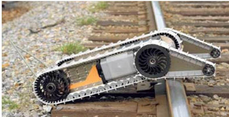
**Figure 33:** A rigid track system encountering a discontinuity [67]
