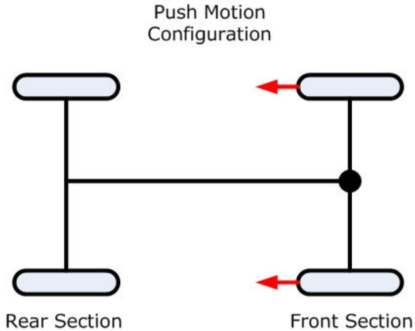
**Figure 104:** "Push" configuration of the two-body vehicle design
