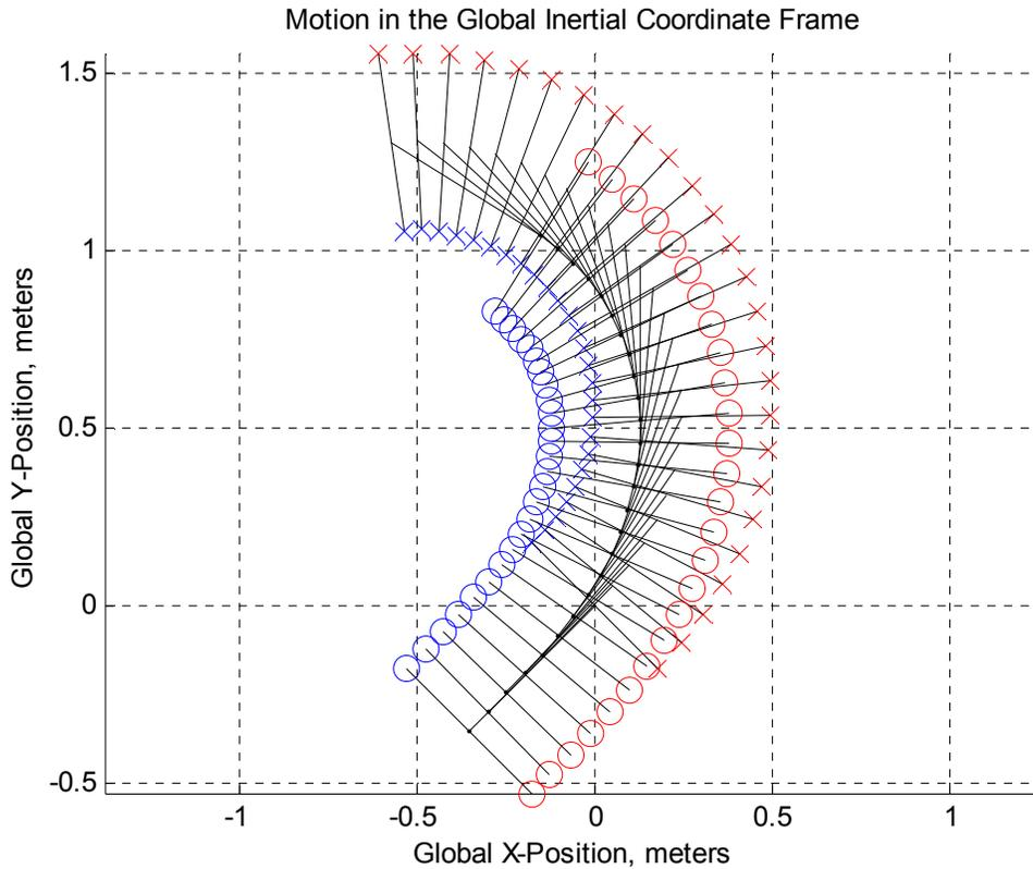
**Figure 40:** Predicted path for the same initial pose as Figure 39 but with differing front wheel velocities.
