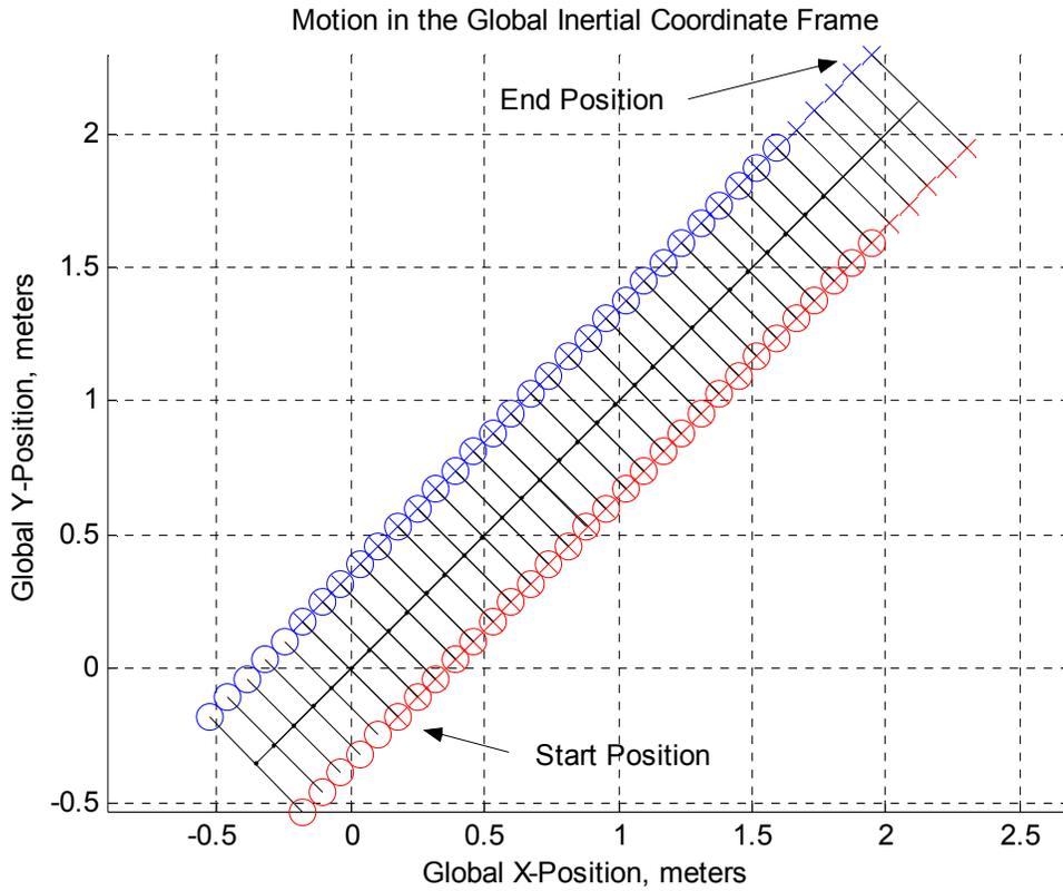
**Figure 39:** Simple case of predicted vehicle path. Red denotes the right side of the vehicle and blue the left. X's indicate the front wheels and O's indicate the rear wheels.
