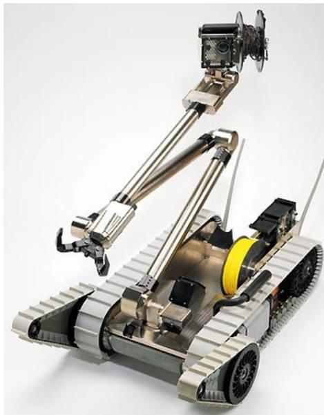
**Figure 14:** iRobot PackBot with EOD manipulator and cable spooler [33]
