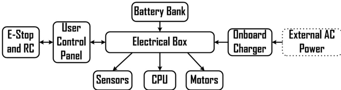
Figure 24: Gemini power system schematic
