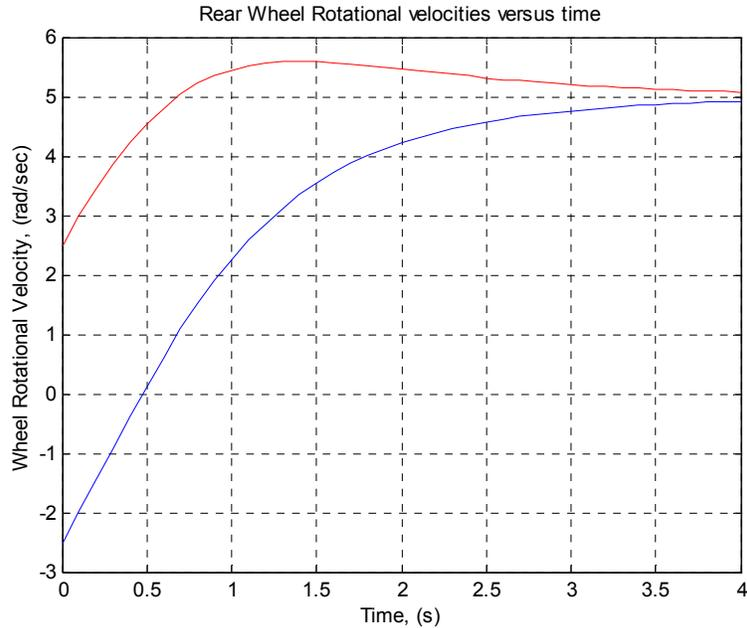
**Figure 97:** Rear wheel velocities for case #3. Red indicated right rear wheel while blue is the left rear wheel.
