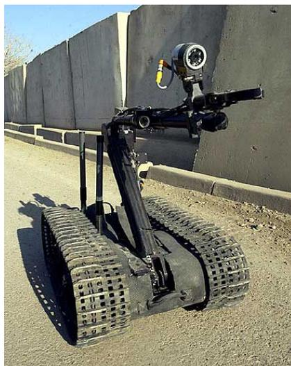
**Figure 15:** Foster-Miller Talon with the gripper manipulator payload [36]
