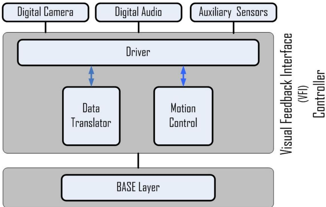
**Figure 52:** VFI controller architecture
