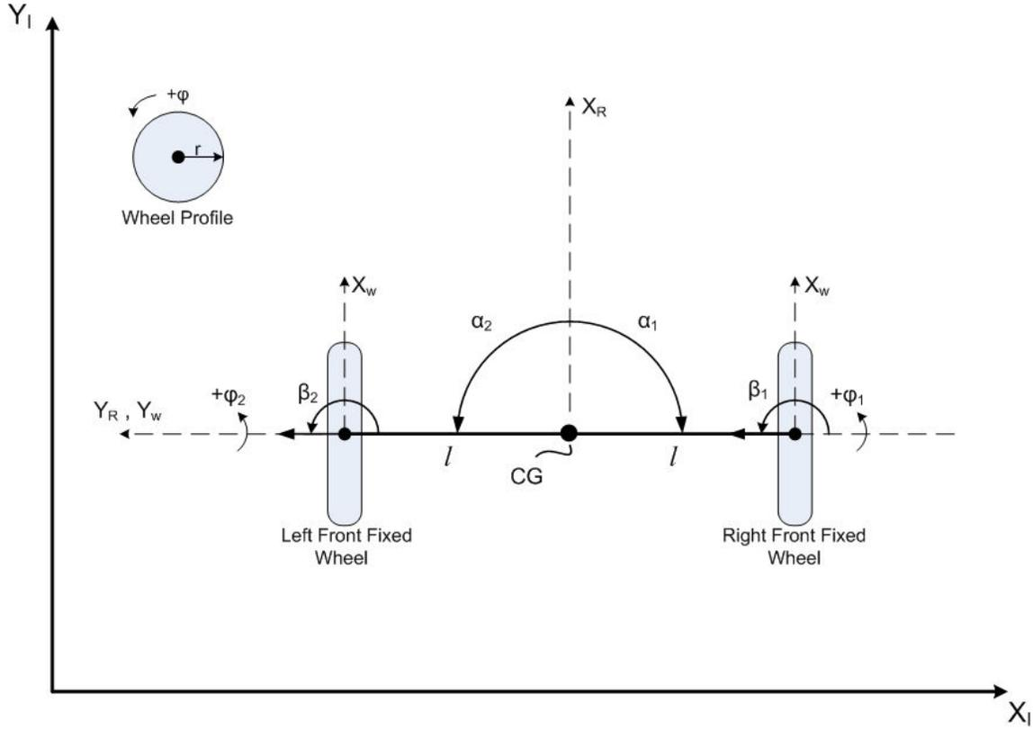
**Figure 36:** Kinematic model of the front section
