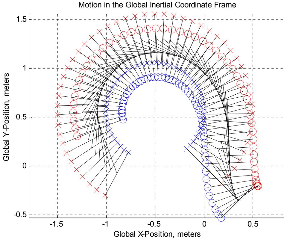
**Figure 41:** Predicted path of vehicle motion highlighting the tendency of the rear section to seek equilibrium with the front section of the vehicle.
