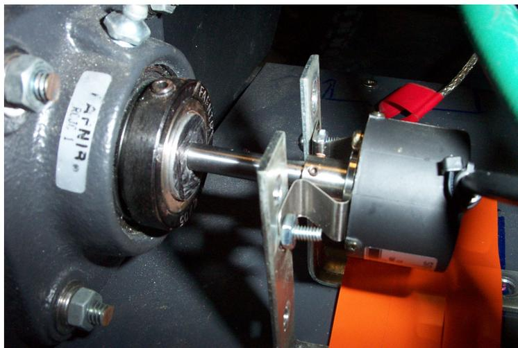
**Figure 74:** Detail of incremental encoder mounting solution
