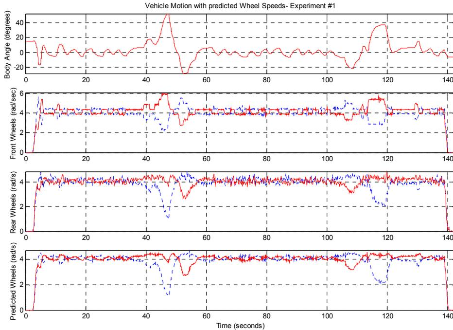
**Figure 81:** Measured vehicle motion with predicted rear wheel speeds
