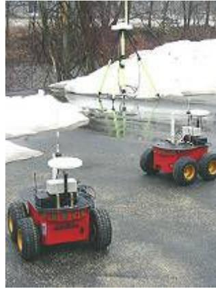
**Figure 21:** ActivMedia Robotics Pioneer3 -AT vehicle platform [46]
