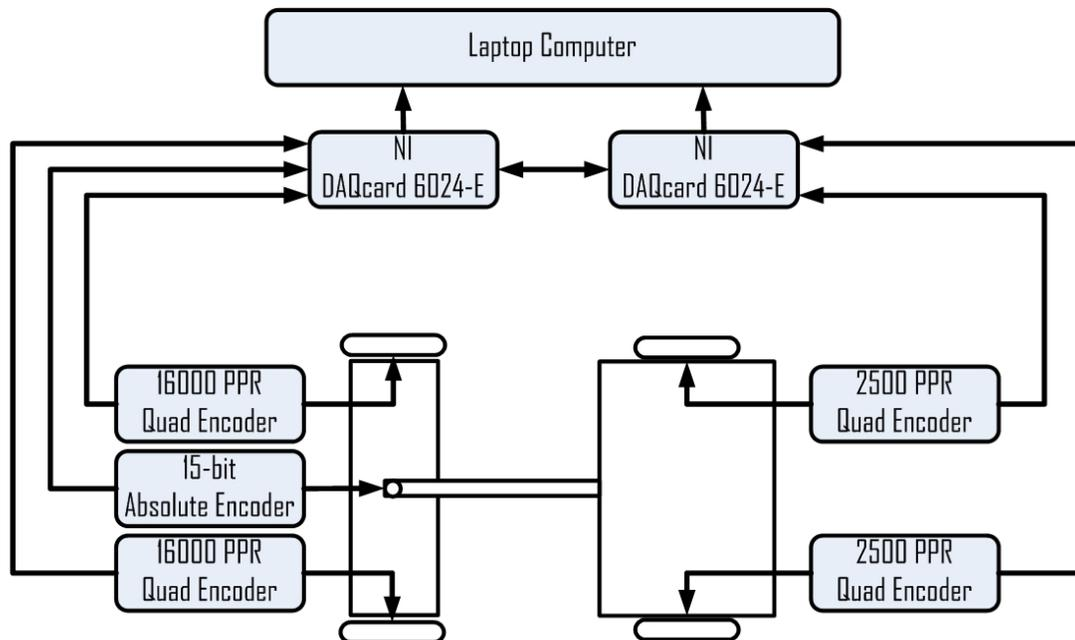
**Figure 71:** Schematic of the instrumentation implemented on Polaris
