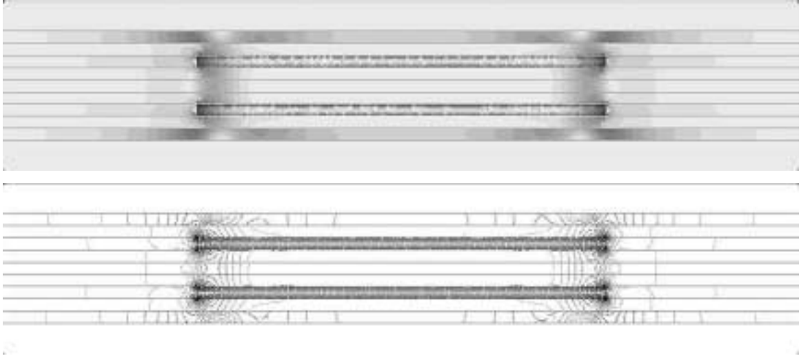
Figure [8] Low permeability magnetic material surrounding coils.
