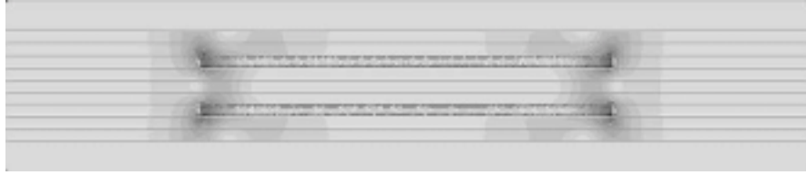
Figure [20] Flux distribution at 2.0 MHz for a single material core, \mu = 220 .
