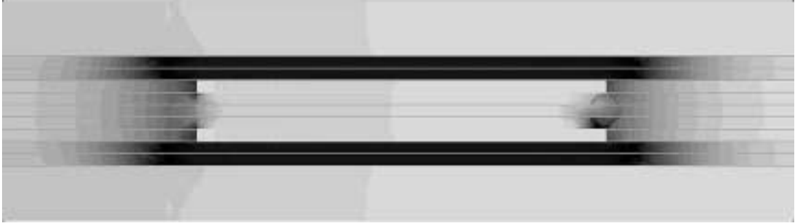
Figure [34] Composite model with a permeability of \mu = 16 substituted into the TL layer.
