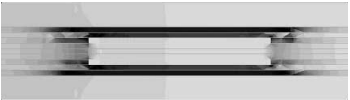
Figure [35] Composite model with a permeability of \mu = 16 substituted into the CL layer.
