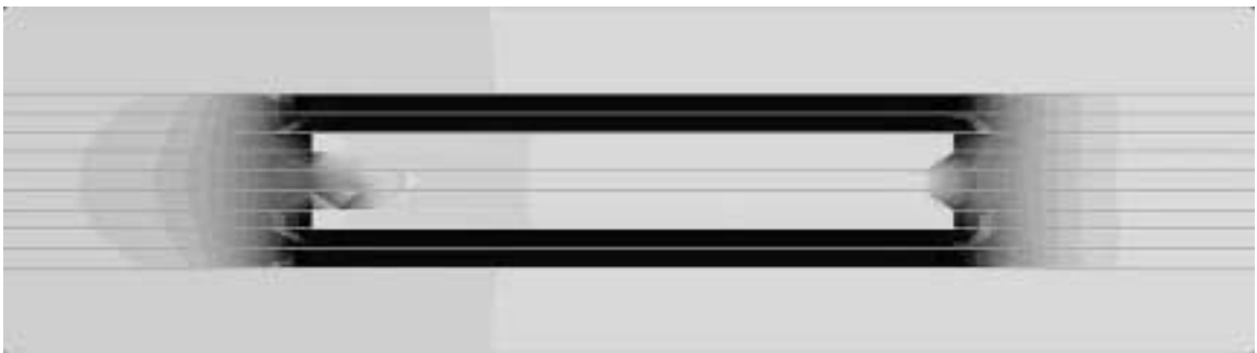
Figure [33] Composite model with a single material core, with a permeability of \mu = 220 .
