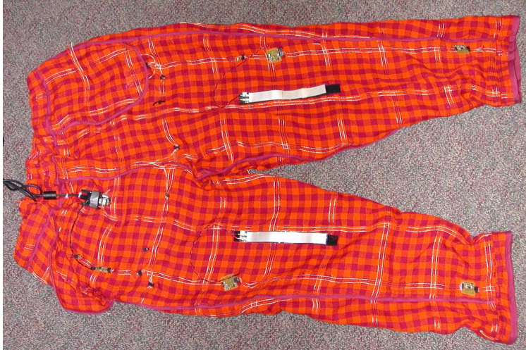
Figure 2.1: E-textile pants for context recognition and gait analysis
