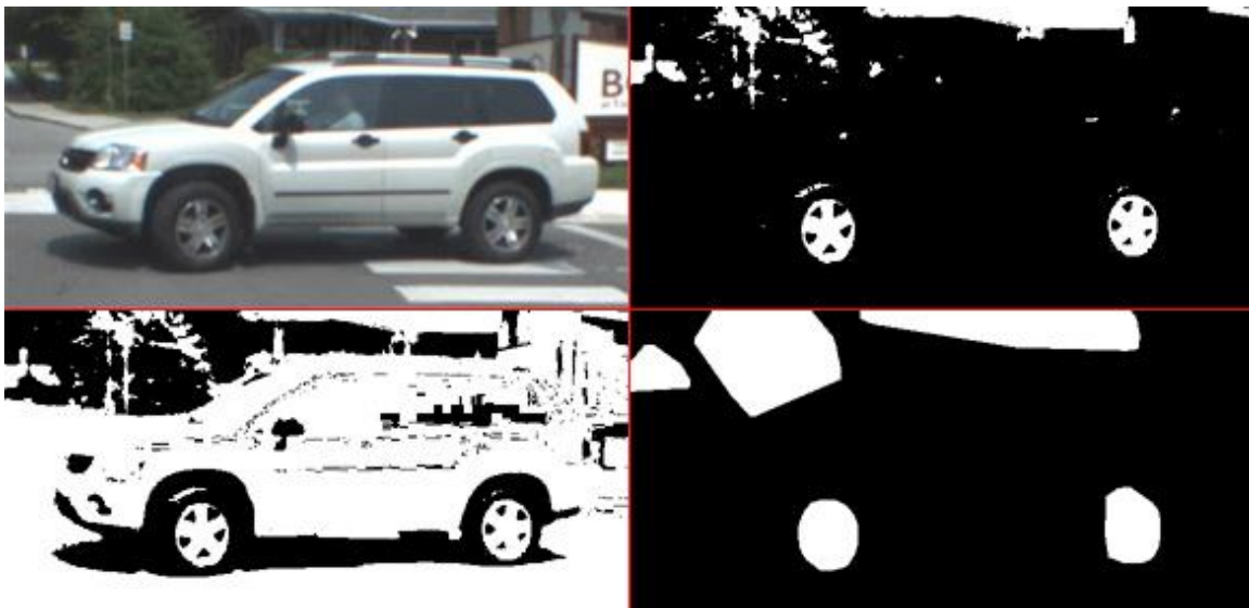
Figure 5-12: Panels showing the HSL region (upper-left), the threshold operation (lower-left), the particles after segmentation and large particle filter (upper-right), and the final particle image (lower-right).
