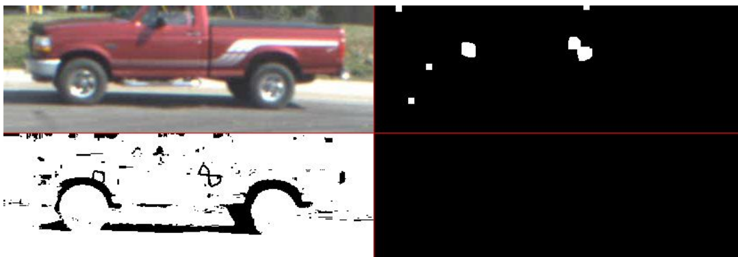
Figure B-22. A red truck observed at a medium distance. Here the lighting conditions are unfavorable again, this time due to the large amount of light. The detector is unable to segment out the hubcap from the rest of the tire.
