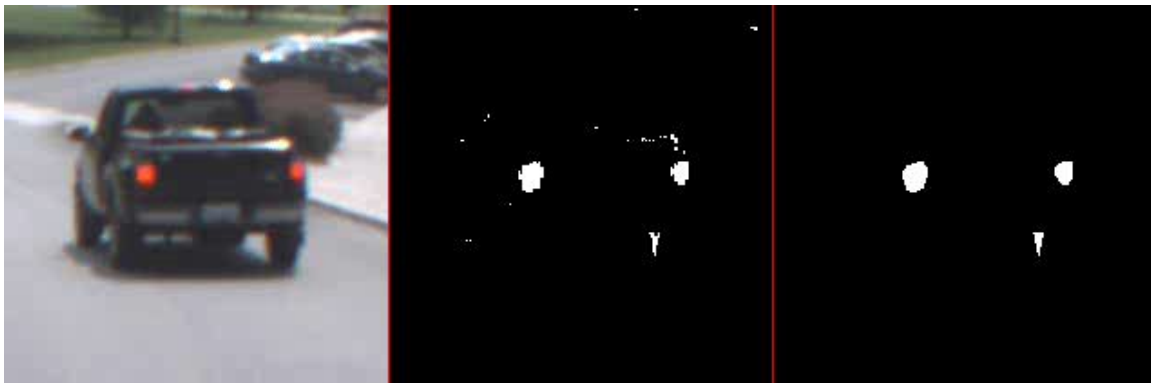
Figure B-2. The same black truck with the brake lights illuminated at an angle. The software again successfully finds the tail lights.
