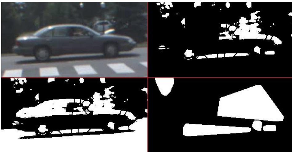
Figure B-20. A grey car observed at a medium distance in poor lighting. In this case even though the hubcaps are able to be segmented, the light area seen under the body is merged with one of the tires. The result is that the software is unable to find a particle match.
