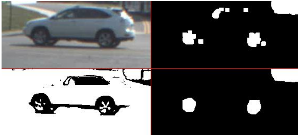
Figure B-19. A white SUV observed at a far distance. Once again the software is successful with the segmentation even at a good distance if the lighting is favorable.
