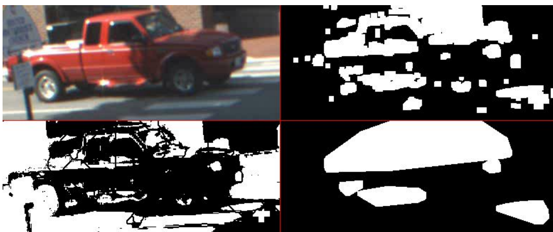
Figure B-23. A red car half in the shadow of a building. The rear tire can not be segmented due to how bright the surrounding tire is, while the forward tire fails due to the low light in the shadow area.
