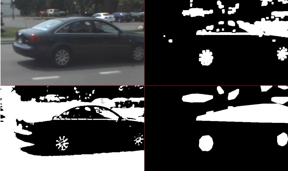
Figure B-24. A blue car observed at a short distance. Even though the entire car is not in the extracted region, the segmentation and subsequent detection succeeds. This figure illustrates how the tire detection software is not as sensitive to the region extraction as the tail light software is due to the location of the tires relative to the edges of the vehicle.
