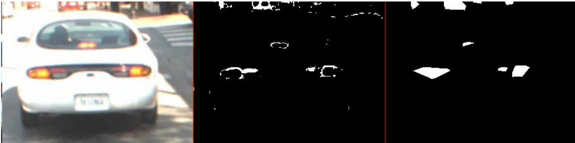
Figure B-8. A white car with tail lights illuminated. The software fails to detect the tail lights based on the area and ratio criteria. This failure is due to the image being extremely bright after coming out of a shaded area, causing the hue of the tail lights to be shifted outside of the threshold range.
