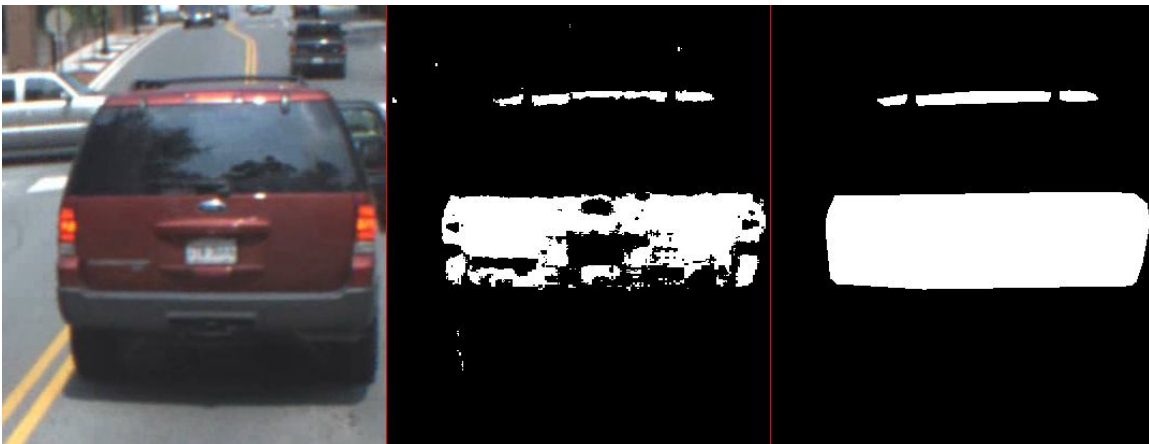
Figure B-9. A red van with tail lights illuminated. The software fails to detect the tail lights due to the red body color. However, the red car detector is able to determine that there is a single large particle in the image that is most likely a red car.
