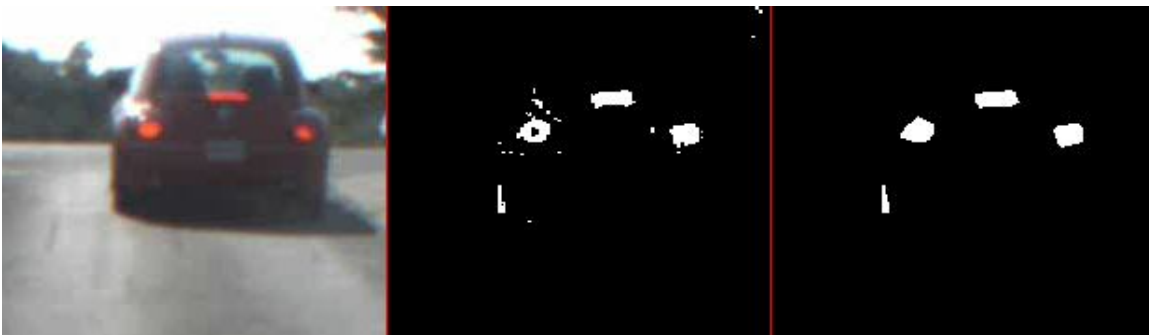
Figure B-4. A red beetle with tail lights illuminated. Although the vehicle is red as well, the shadows on the vehicle body allow the tail lights to be segmented and successfully detected.
