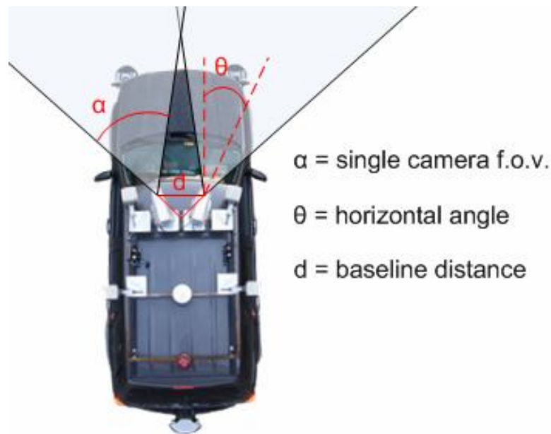
Figure 5-4: Values used to determine the vision systems field of view and blind spot.
