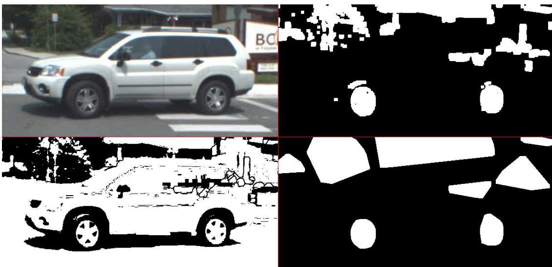
Figure B-15. A white SUV observed at a short distance. The detector is able to find the tires even with the slight deformation to the rear tire.
