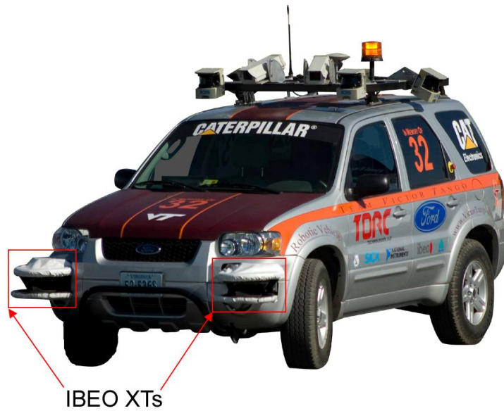
Figure 4-2: The IBEO XT units mounted on the front corners of Odin. The A0 unit is mounted at the center of the rear bumper and can not be seen in this figure.
