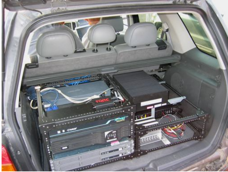
Figure 2-3. The power and computing systems mounted in the rear of Odin. The two servers Bill and Linus can be seen mounted on the bottom-left corner of the rack.
