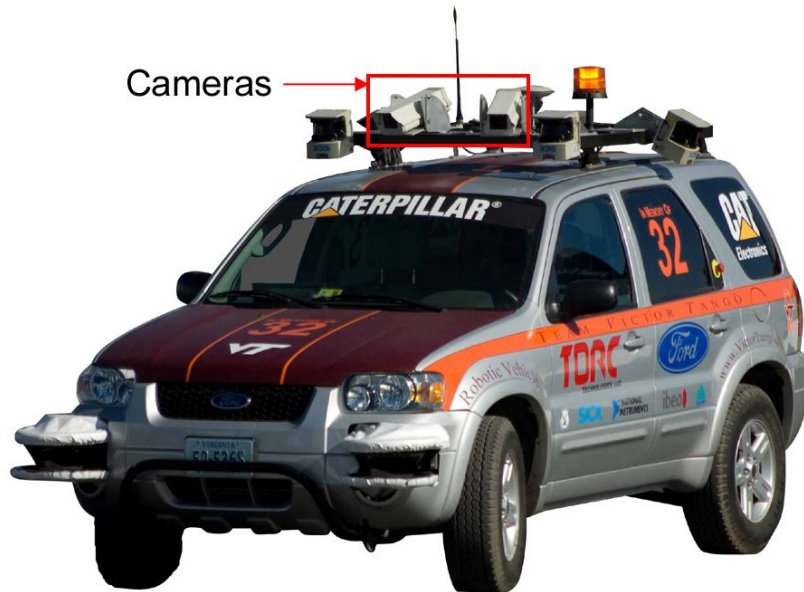
Figure 5-3: The CCD cameras mounted on the top of Odin’s roof rack.
