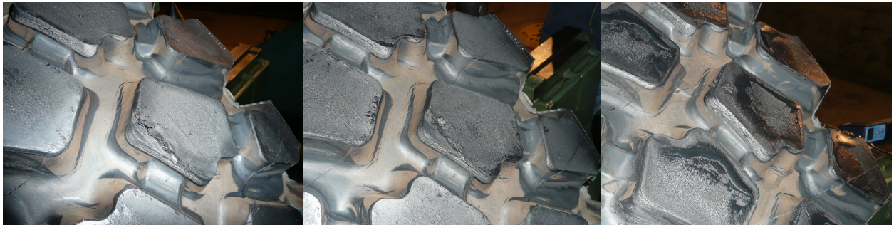
Figure 3.9. Tread wear on studied tire. From left to right: post 20 mph, post 40 mph, post 65 mph
