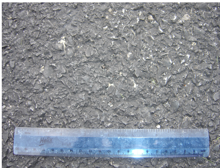
Figure 4.9. Dry asphalt driving surface used as a baseline for the off-road testing
