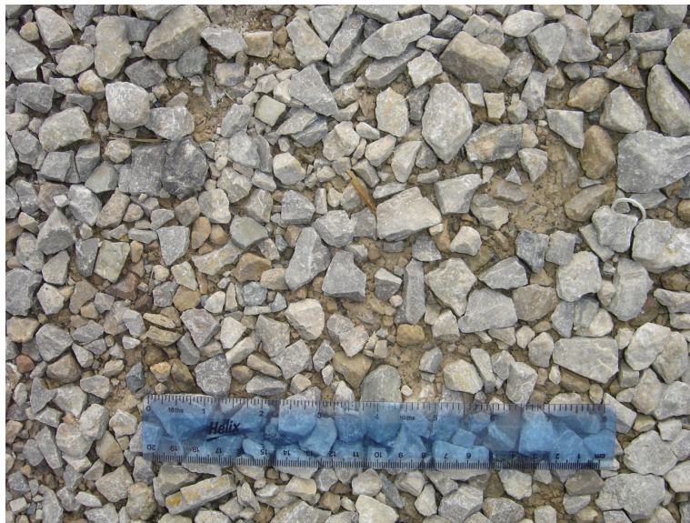
Figure 4.11. Gravel driving surface used for off-road tire testing
