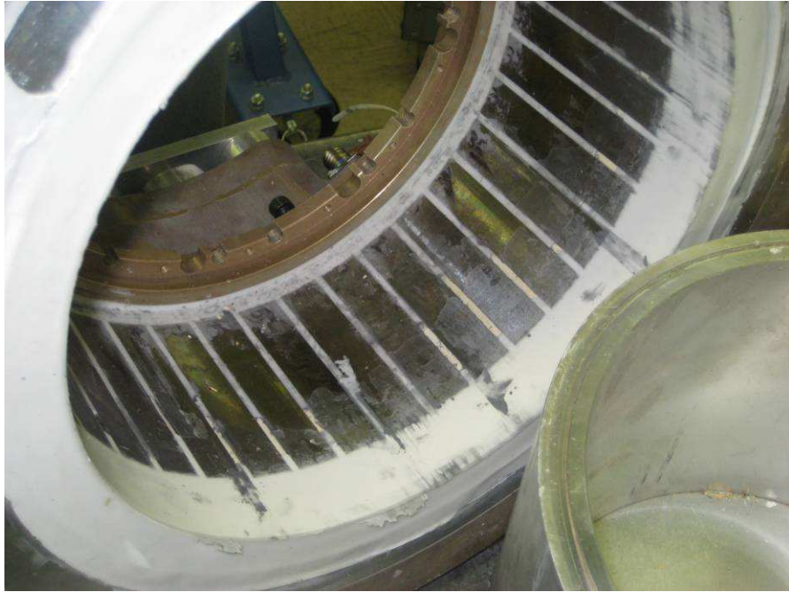
Figure 31 - Encapsulation Voids, "Motor B" Inner Diameter
