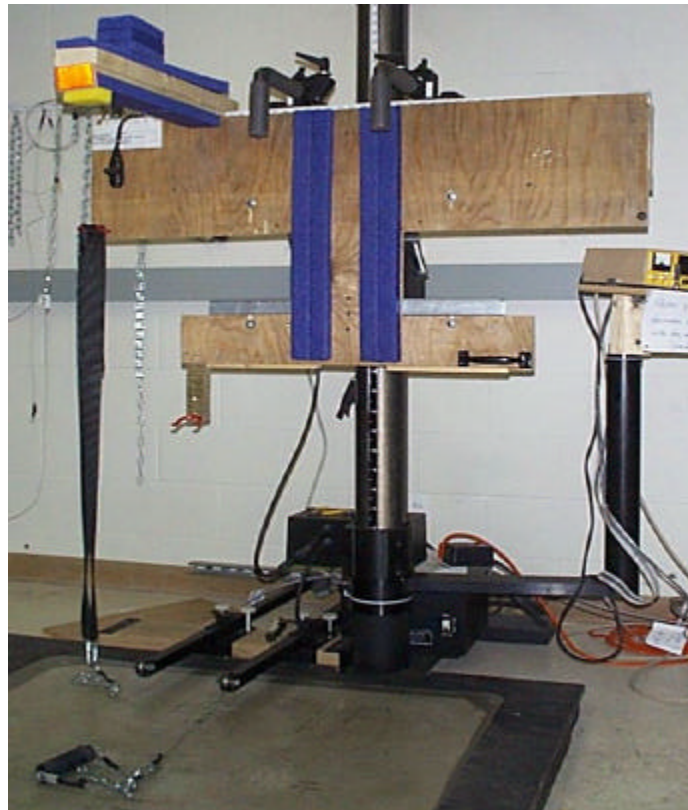
Figure 3. Fixture for lumbar MVC performance.
