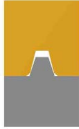
Figure 3.4-1. CAD model showing the teeth designed to hold the material.
