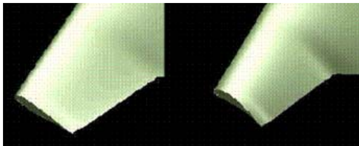
Figure 1.3-4. A morphing wing with different camber configurations. The camber design on the left is with a “normal” camber, while the wing design on the right has an extreme camber shape [Pettit].
