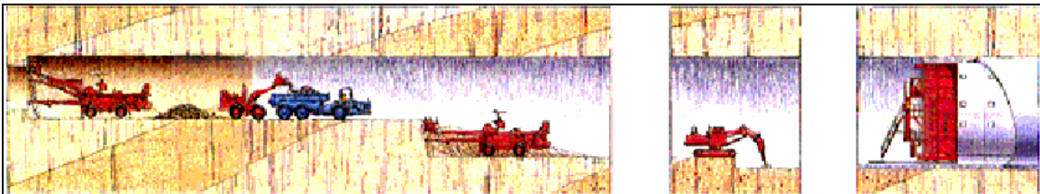
b: Top heading excavation and support followed by bench excavation and support. A short invert stage is left to be excavated last. Finally a water proof geomembrane is installed and a “traveling shutter” (formwork shield) is used for final (secondary) support installation.
