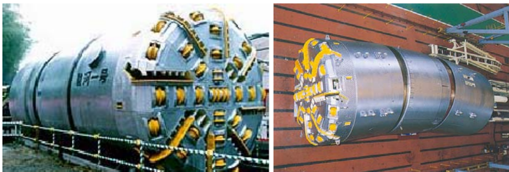
Figure 4.7 a,b: The triple shield TBM used at the Shimizu site.
