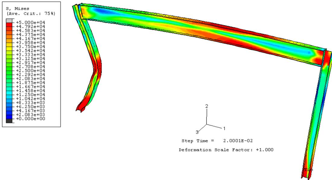
Fig. 3.19. Sample of von Mises stress distribution in the portal frame subjected to a 4,000 psi blast load at time  $t = 20$  msec
