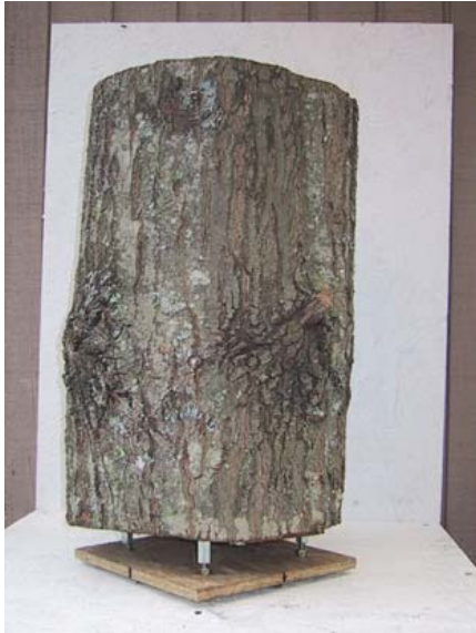
Figure 4. Setup for photographing and measuring sample log sections.
