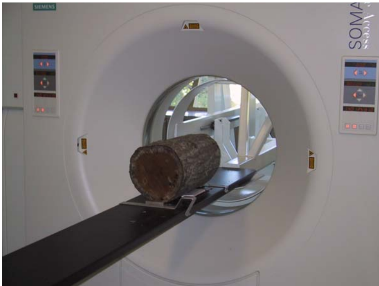
Figure 5. Example CT scanning setup for log section samples.
