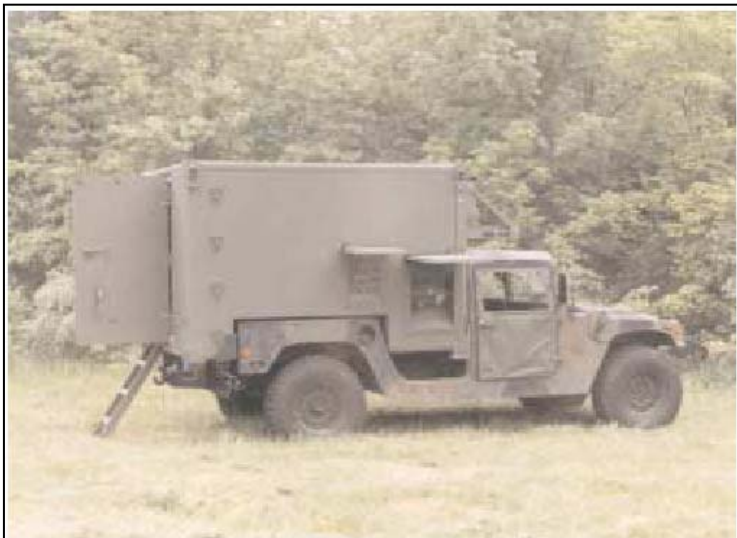
Figure 2.7: A US Army truck configured with the Digital Topographic Support System -Deployable
