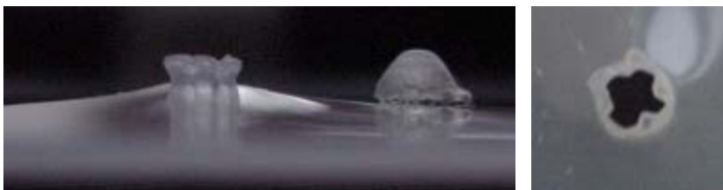
Figure 4-2 LDPE punctures—healing did not occur. Side view (left) and back view (right). The cap of film ejected with the projectile can be seen in the side view image.
