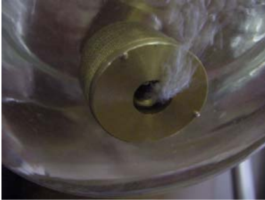
Figure 6-2 The sample film is mounted in the window of the test fixture. Upon increased air pressure, failure of the puncture site is indicated by air bubbles escaping into the water bath.
