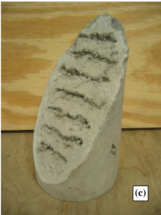
Figure 4.13: Slant Cylinder Concrete Surface Preparations: Smooth (a), Exposed Aggregate (b), Raked (c), and Raked and Sand Blasted (d)
