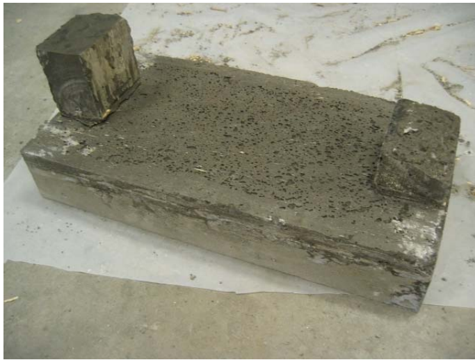
Figure A8: Set ® 45 Hot Weather extended (8) Haunch Flow Mockup
