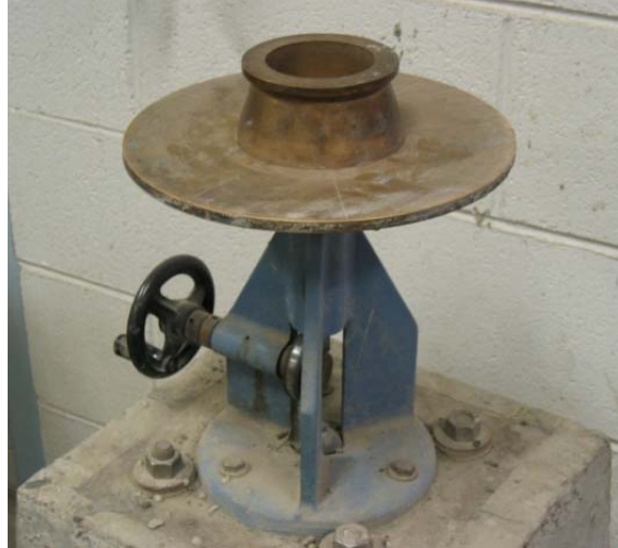
Figure 4.8: Truncated Flow Cone and Drop Table
