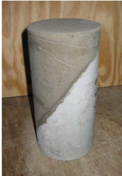
Figure 4.14: Completed Slant Shear Cylinder
