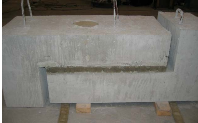
Figure 4.19: Complete Push-Off Specimen with Grouted Interface
