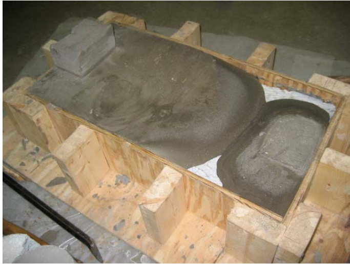
Figure A1: ThoRoc ® 10-60 (1) Haunch Flow Mockup
