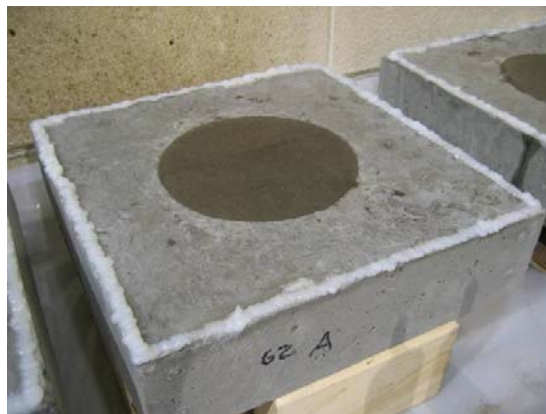
Figure 4.7: Shear Pocket Specimen with Water Ponding
