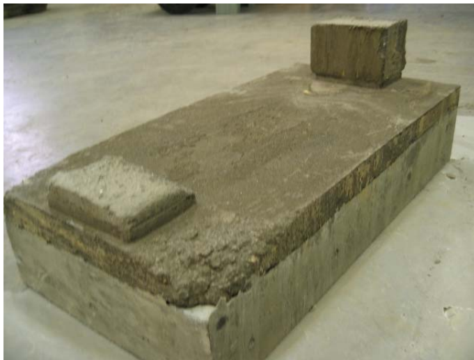
Figure A4: SikaQuick® 2500 extended (6) Haunch Flow Mockup
