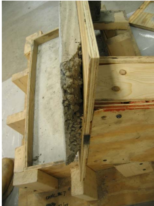
Figure A6: Five Star ® Patch extended (7) Haunch Flow Mockup
