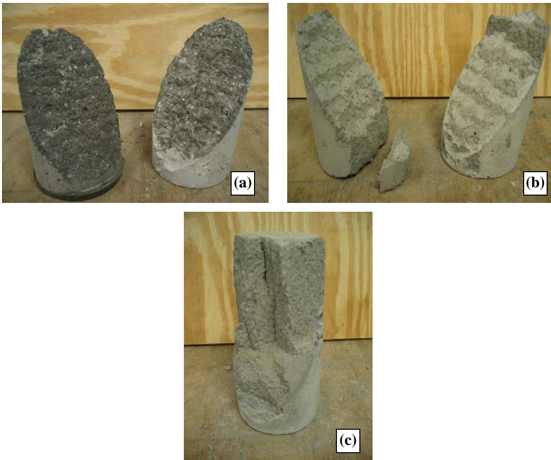
Figure 5.11: Slant Shear Cylinder Failure Modes
