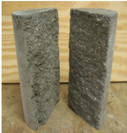
Figure 4.2: Typical Split Cylinder Specimen After Testing per ASTM C 496
