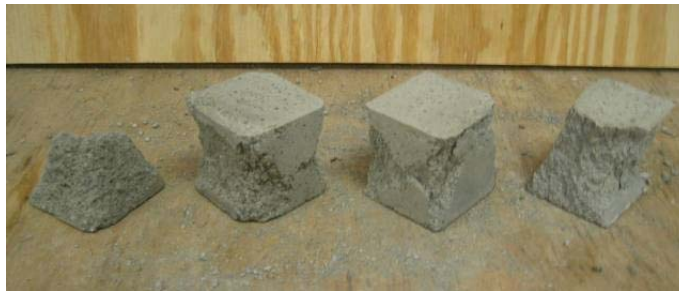
Figure 4.1: Typical 2 in. Cube Specimens After Testing per ASTM C 109
