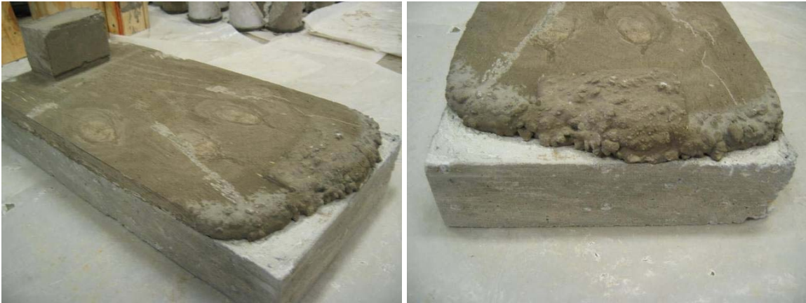
Figure A2: ThoRoc ® 10-60 extended (5) Haunch Flow Mockup
