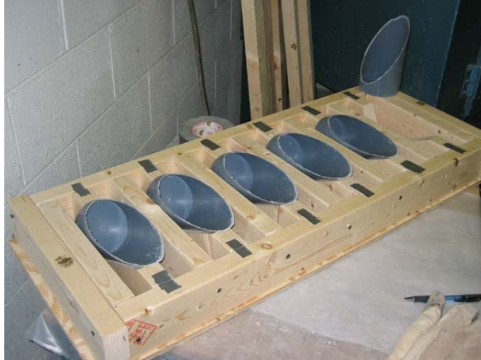
Figure 4.12: Sliced 4 in. x 8 in. Cylinders for Slant Cylinder Tests
