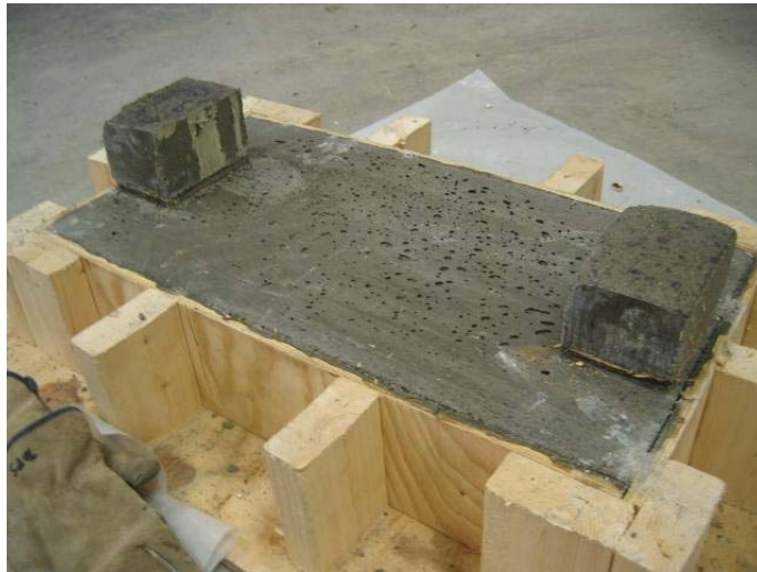
Figure 5.9: Set ® 45 Hot Weather (4) Flow Through Haunch Mockup
