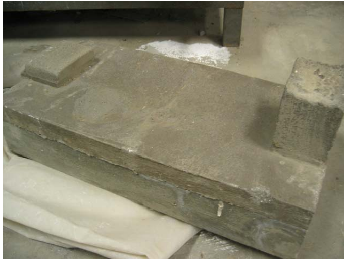
Figure A3: SikaQuick® 2500 (2) Haunch Flow Mockup
