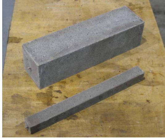
Figure 4.5: Neat Mortar (bottom) and Aggregate Extended Mortar Shrinkage Bars
