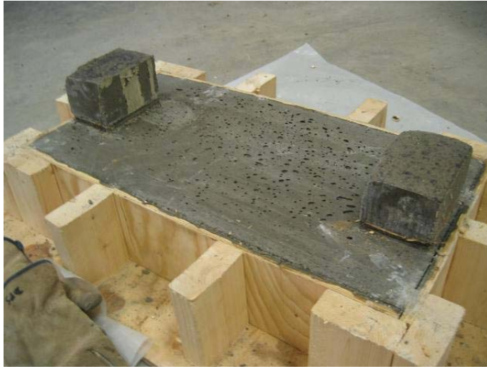
Figure A7: Set ® 45 Hot Weather (4) Haunch Flow Mockup
