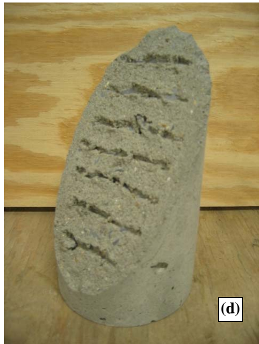
Figure 4.13: Slant Cylinder Concrete Surface Preparations: Smooth (a), Exposed Aggregate (b), Raked (c), and Raked and Sand Blasted (d)
