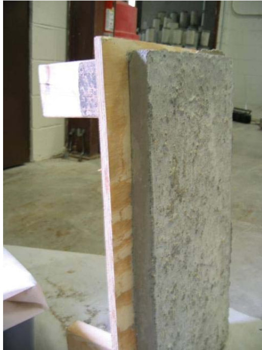
Figure A5: Five Star ® Patch (3) Haunch Flow Mockup
