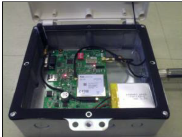
Figure 3: Bluetooth unit chipset design with GPS+GSM [4]
