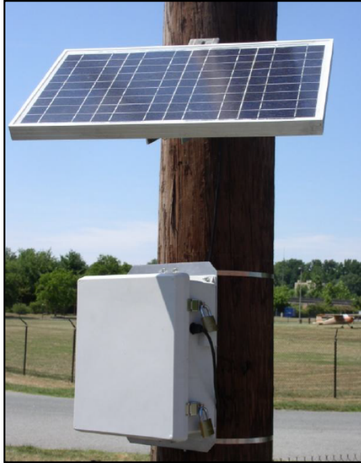
Figure 4: Bluetooth Unit with Solar Energy Capability [17]
