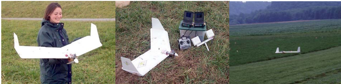
Fig 4.1: (Left) the UAV, (Middle) the UAV with the remote control, video system, and antennae, and (Right) the UAV flying low over an alfalfa field at the Virginia Tech Kentland Research Farm, Montgomery Co., VA
