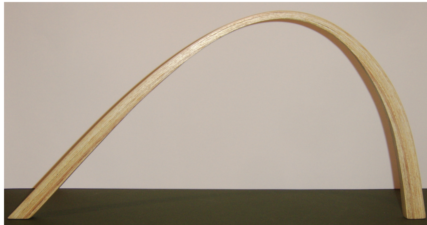
Fig. ii-1 Glue-Laminated Arch (Scale Model) (Photo By Author)
