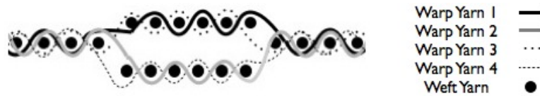
Figure 5.5: Double-weave cross section
