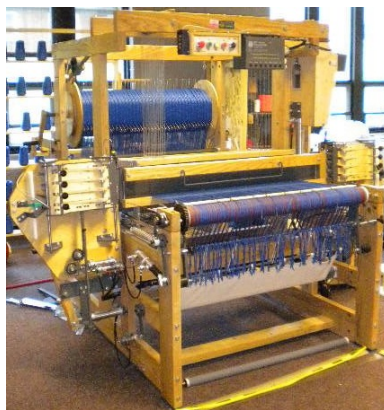
Figure 2.2: 40-inch wide AVL 24-harness Industrial Dobby Loom
