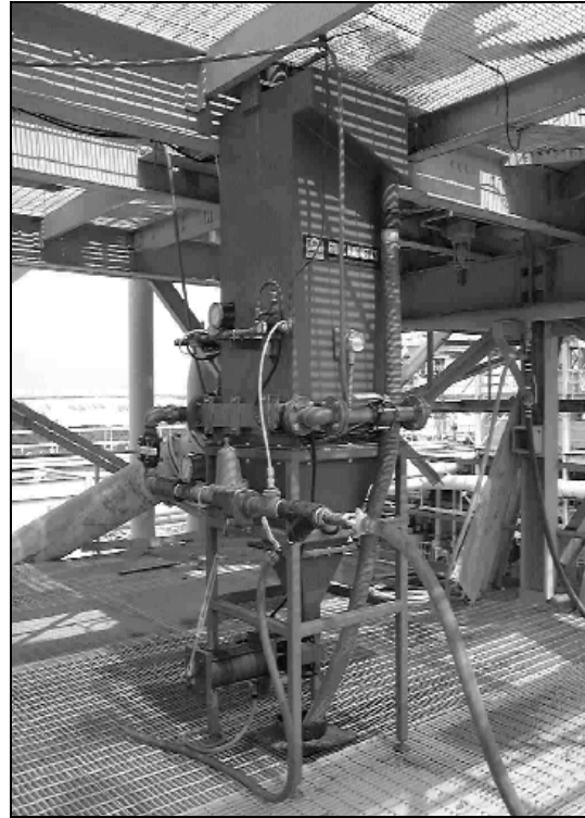
Figure 7. Photograph of the Pilot-Scale HydroFloat Separator.
