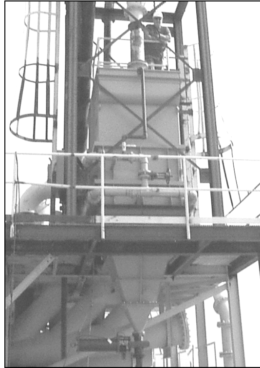
Figure 5. Photograph of the 5 ft x 5 ft CrossFlow Classifier.
