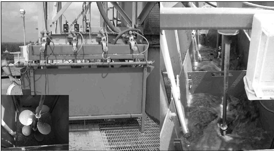
Figure 6. Photograph of the Stirred-Tank Conditioner.
