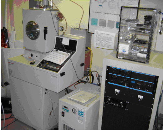
Figure 2.24 RF sputter for deposition of thin metal film
