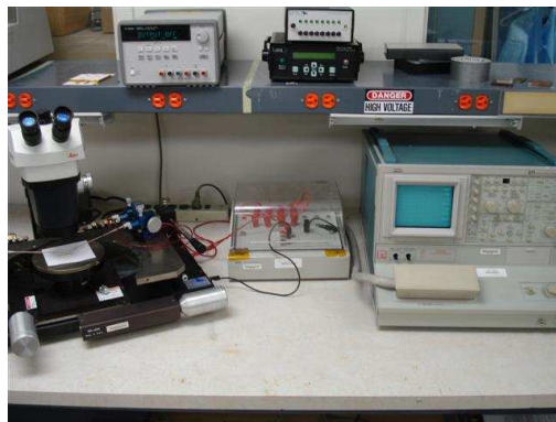
Figure 2.34 Curve tracer for measuring current and voltage
