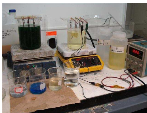
Figure 2.21 The setup of nickel/silver electroplating
