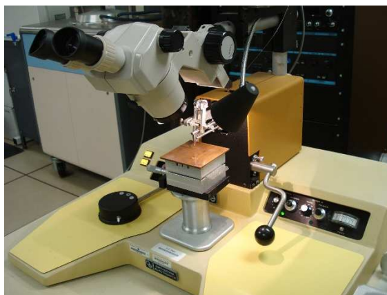
Figure 2.19 Wedge wire bonder
