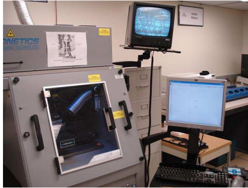
Figure 2.9 Laser cutting machine to cut tape and ceramic
