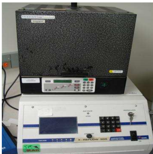
Figure 3.5 Baking oven for curing epoxy
