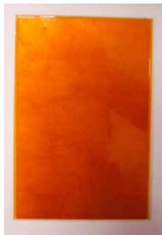
Figure 2.10 DBC panel covered with Kapton® tape
