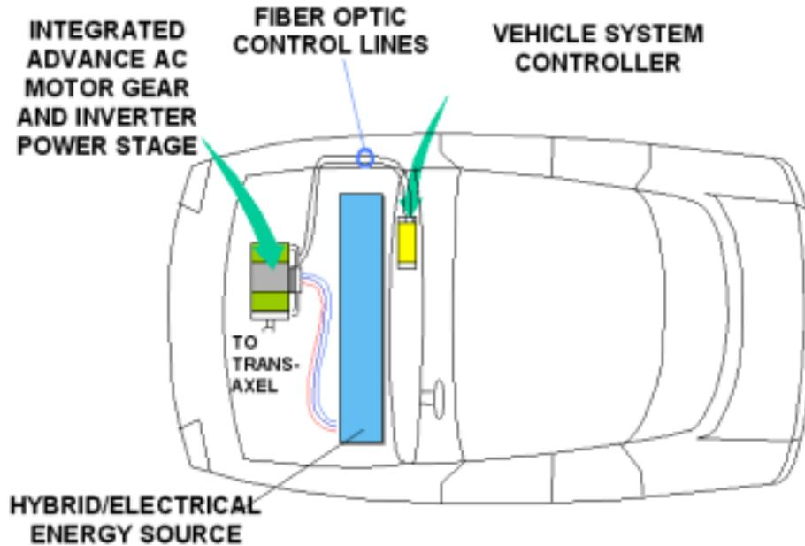
**Figure 9 Motor Drive Integration into Electric Vehicle**
