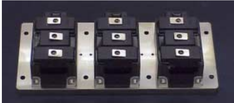
Figure 34 IGBT Modules Soldered to Base Plate
