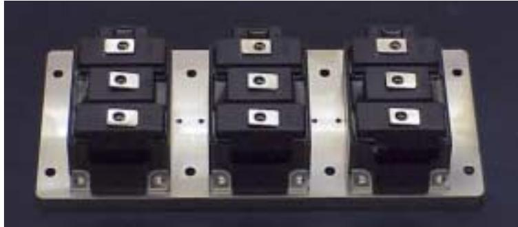
**Figure 34 IGBT Modules Soldered to Base Plate**
