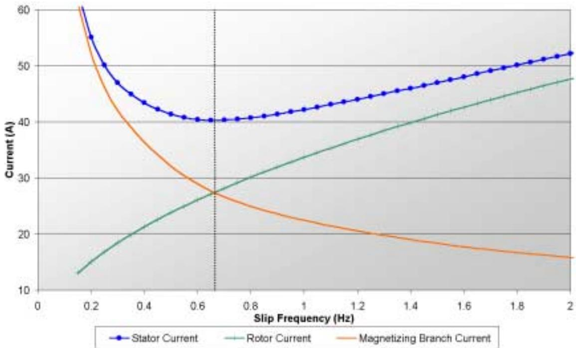
**Figure 20 Various Motor Currents - 3000RPM 5ft-lb**
