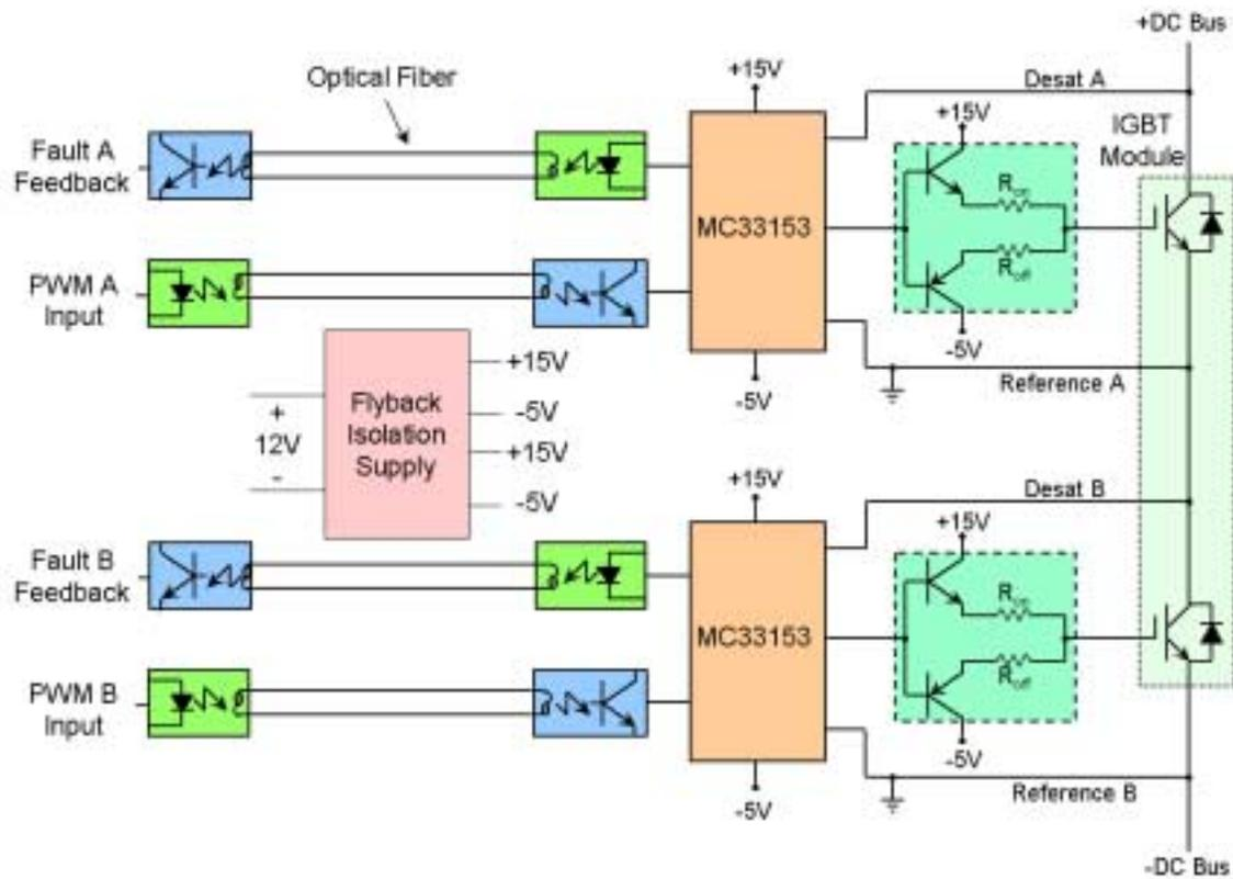
**Figure 28 Block Diagram of Gate Drive Circuit**
