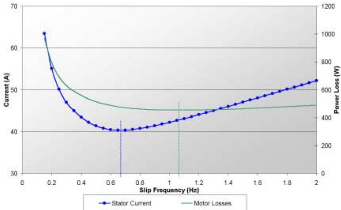
Figure 12 Stator Current and Motor Losses - 3000RPM 5ft-lb
