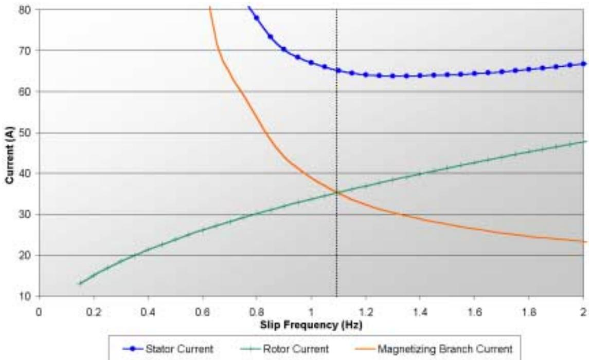
Figure 22 Various Motor Currents - 10000RPM 5ft-lb
