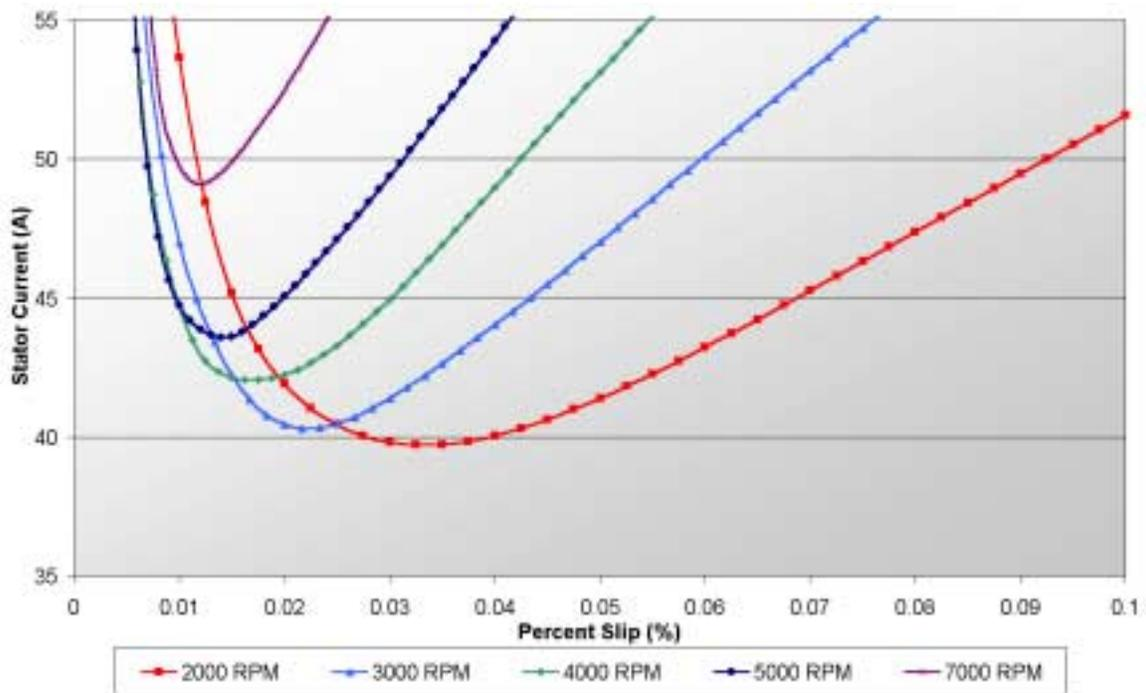
Figure 19 Maximum Torque per Ampere vs Percent Slip
