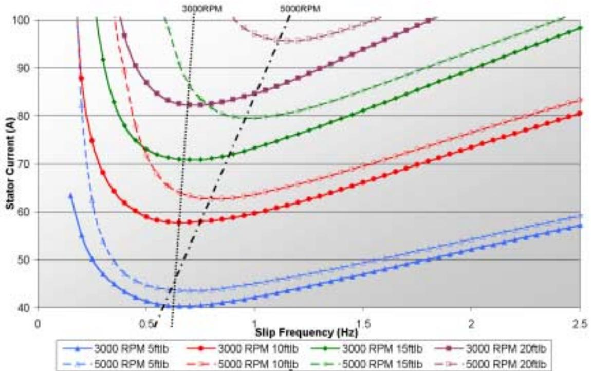
**Figure 17 Maximum Torque per Ampere - Two Rotor Speeds**
