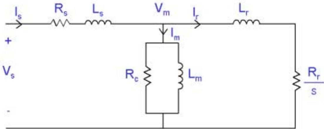
**Figure 10 Equivalent Circuit of an Induction Motor**
