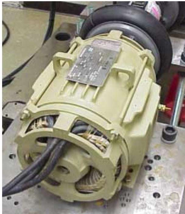
Figure 24 Prototype Induction Motor for Traction Drive
