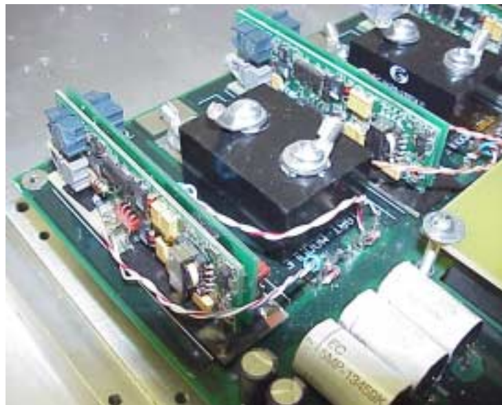
Figure 33 Integrated Gate Drivers and Capacitors
