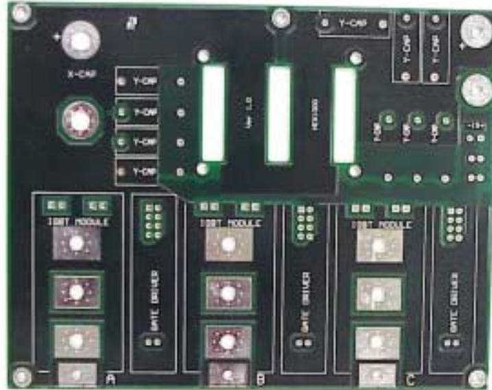
**Figure 27 Inverter PCB Integrated BusBar**
