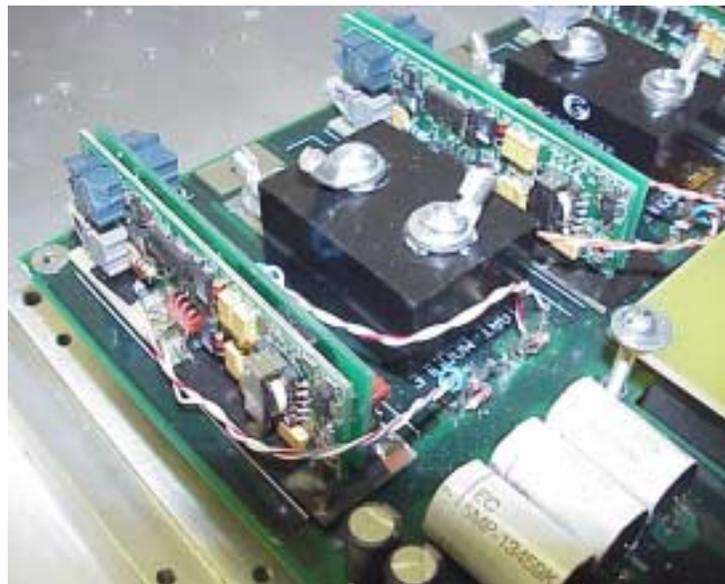
Figure 33 Integrated Gate Drivers and Capacitors
