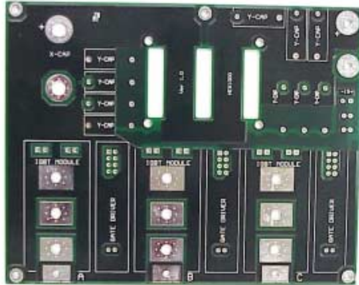
Figure 27 Inverter PCB Integrated BusBar
