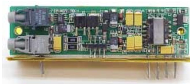
**Figure 29 Gate Drive Module**
