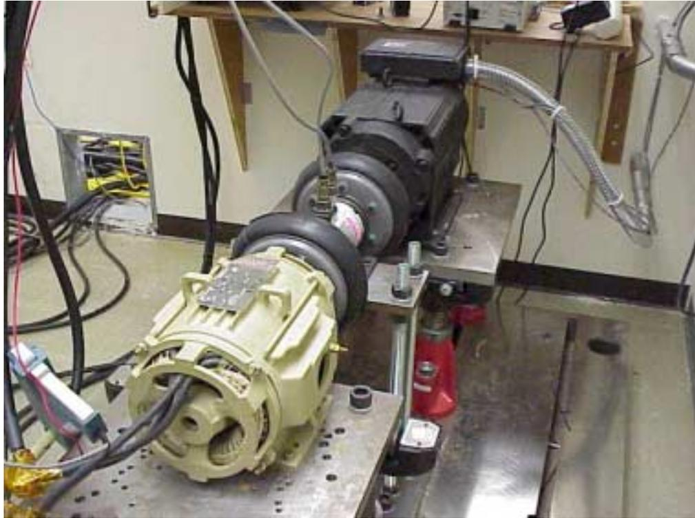
**Figure 36 Traction Motor Drive Connected to Dynamometer**
