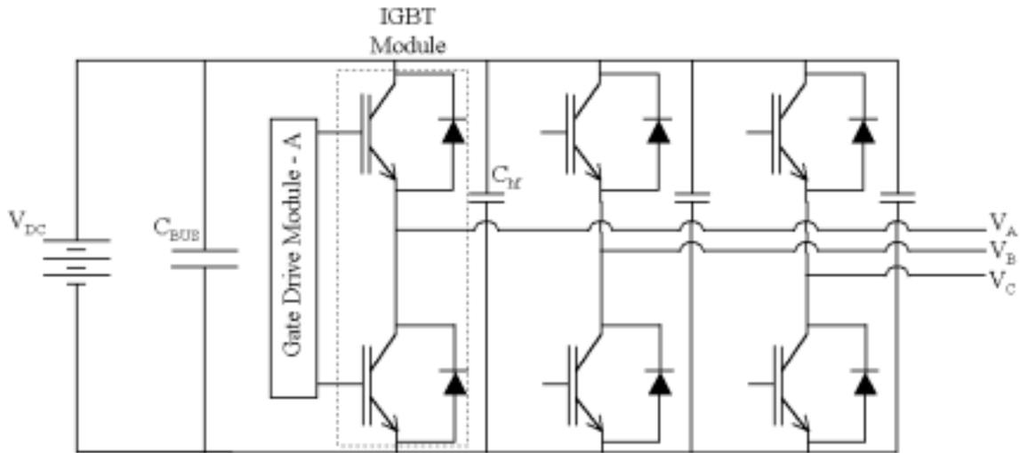
**Figure 26 Motor Drive Inverter Power Circuit Schematic**
