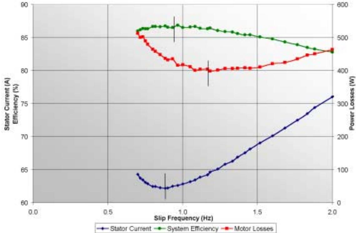
Figure 42 Maximum System Efficiency  $n_s=3061$  T=10ftlb
