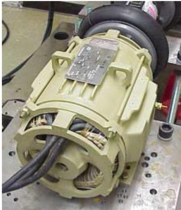
**Figure 24 Prototype Induction Motor for Traction Drive**
