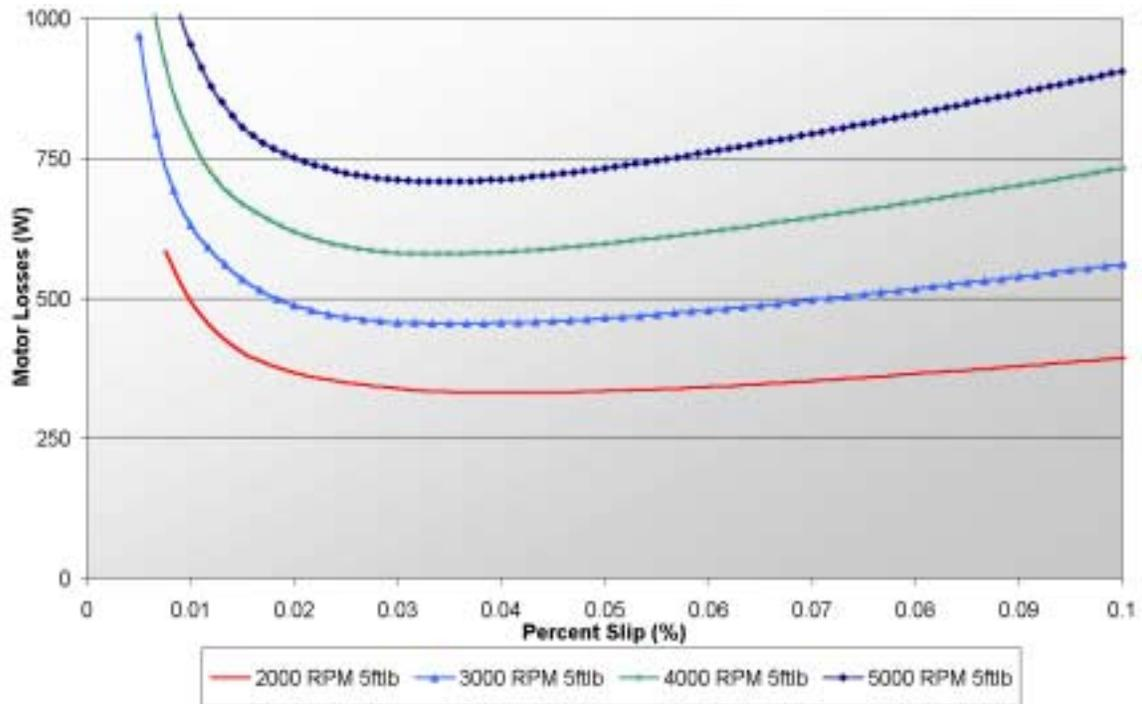
**Figure 15 Motor Losses vs. Percent Slip - 5ft-lb**
