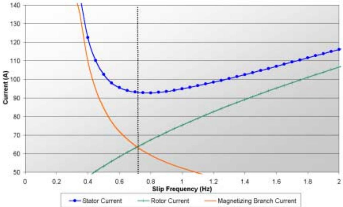
Figure 21 Various Motor Currents - 3000RPM 25ft-lb
