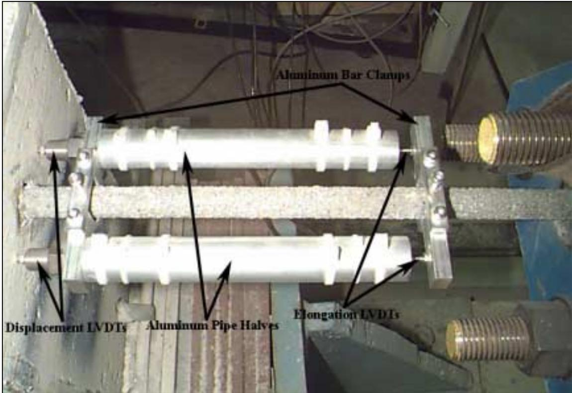
**Figure 3.16: Loaded end bar rig and LVDTs.**
