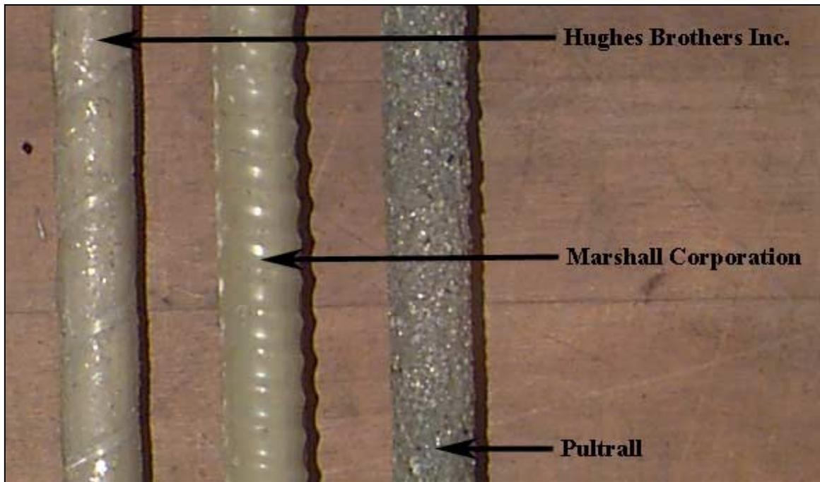
**Figure 3.1: Examples of the three manufacturers' bars.**
