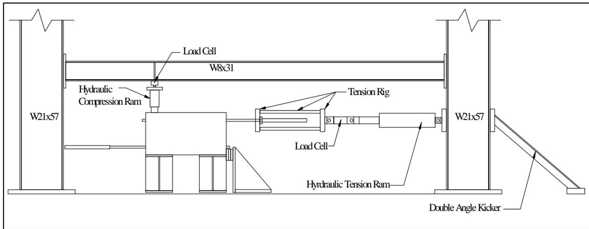
**Figure 3.11: Test frame and equipment**
