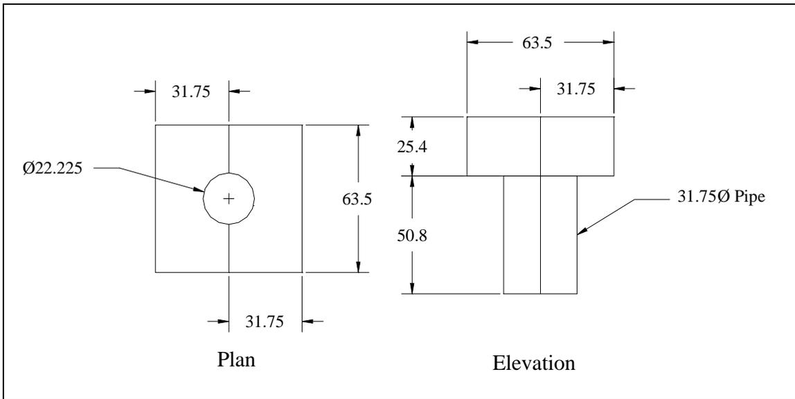
**Figure 3.13: Washer plate for the tension rig.**
