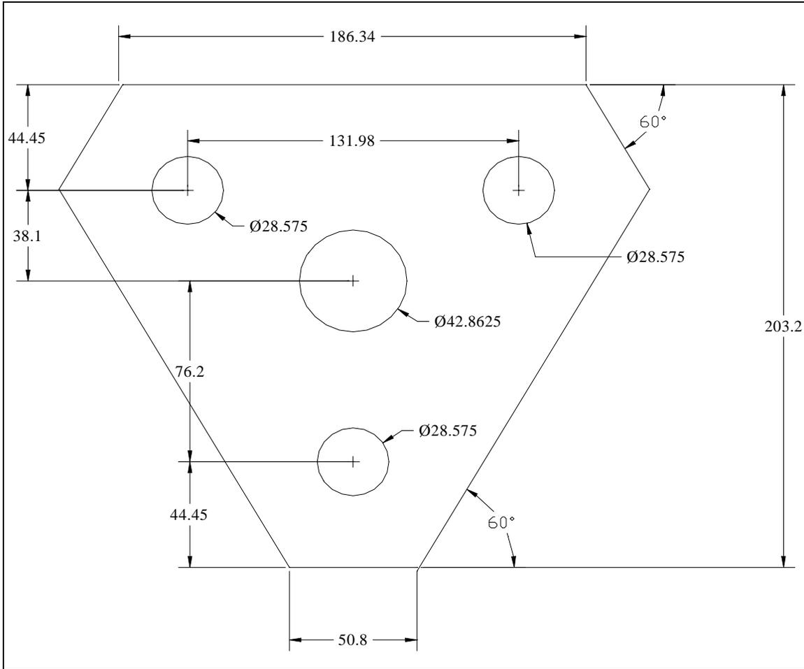
**Figure 3.12: Anchor plate for the tension rig.**
