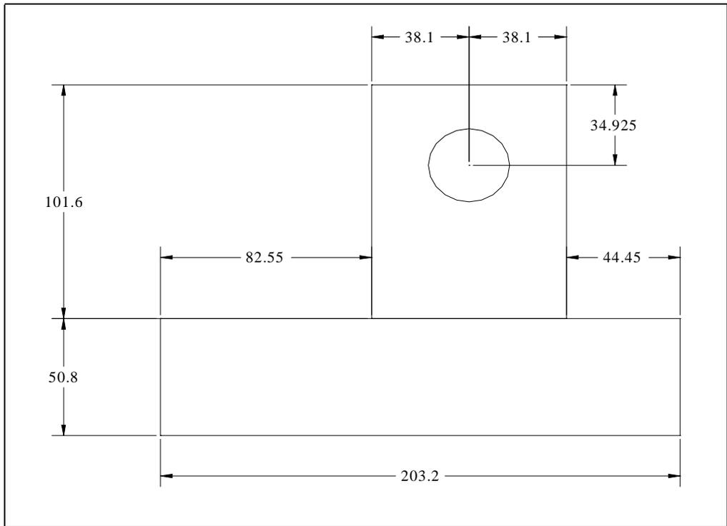
**Figure 3.15: Elevation view of the ram plate for the tension rig.**
