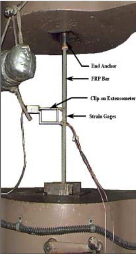
**Figure 3.3: Typical tensile test setup.**
