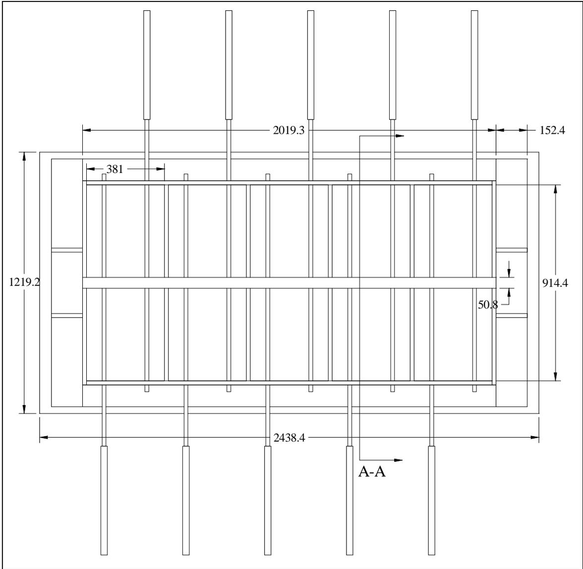
**Figure 3.6: Typical gang form dimensions (plan).**
