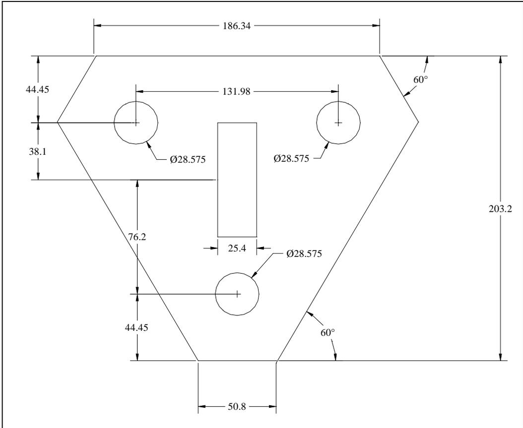
**Figure 3.14: Plan view of the ram plate for the tension rig.**
