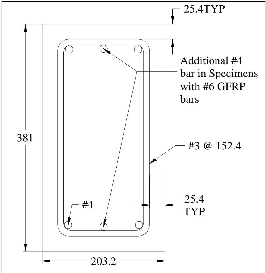
**Figure 3.9 Shear Reinforcement cross-sections.**
