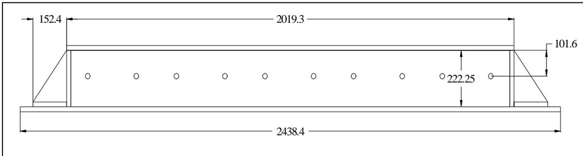
**Figure 3.7: Typical gang form dimensions (elevation view).**
