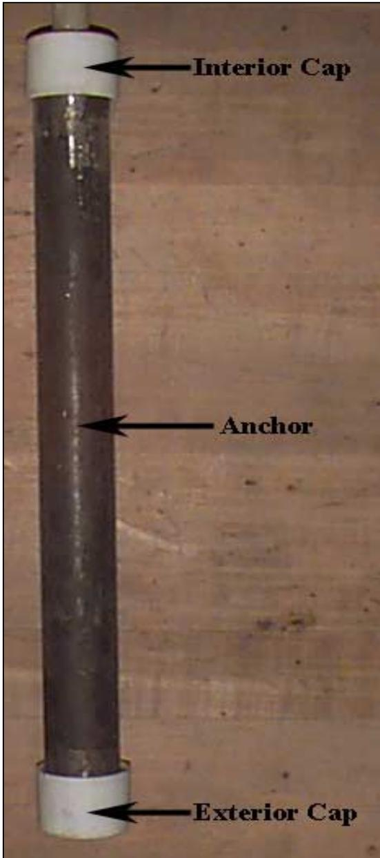
**Figure 3.2: Typical end anchor.**
