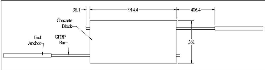
**Figure 3.4: Typical specimen dimension (elevation).**
