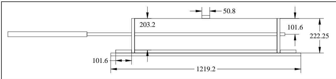
**Figure 3.8: Typical gang form dimensions (elevation view, section A-A).**
