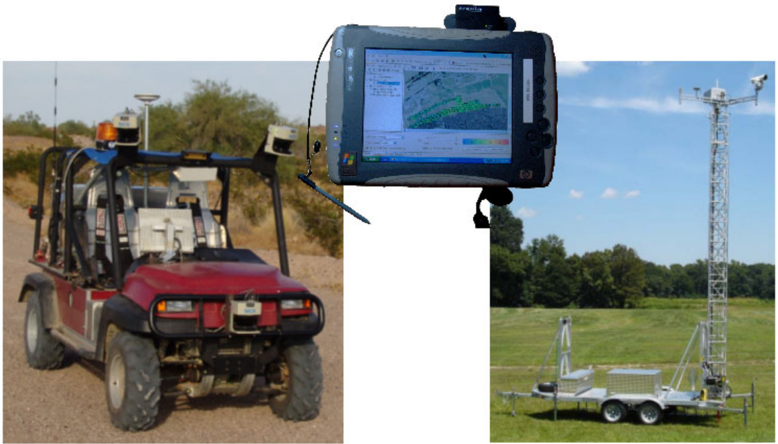
Figure 4.1: Ekahau Site Survey Hardware. UGV Rocky (left), Tablet PC running Ekahau (center), and MIP (right).
