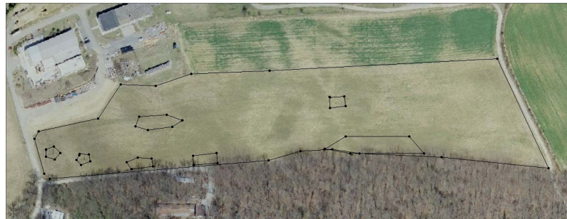
Figure 5.12: Vehicle boundary (perimeter of the field) and obstacles overlaid on the test field.
