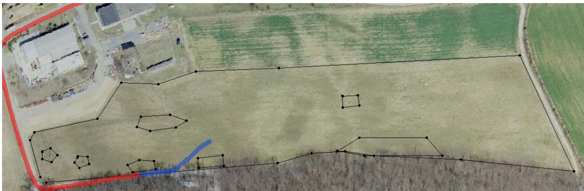
Figure 5.16: Vehicle Boundary Evaluation Results. As the path of the vehicle crosses the boundary line, it changes from red (out of bounds) to blue (in bounds).
