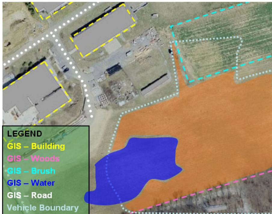
Figure 5.19: Illustration of Example GIS Data. The aerial photo of the test field has been overlaid with building perimeters, tree line of the woods, difficult-to-traverse brush, bodies of water, and roads. Also shown is the predetermined vehicle boundary that the communication subsystem must operate.
