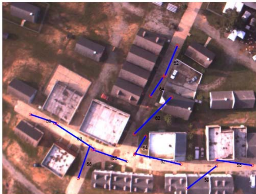
Figure 2.1: “Preliminary experimental radio connectivity map for the Fort Benning MOUT site” [2]
