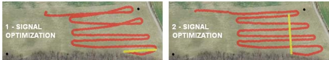
Figure 4.9: NetStumbler Site Survey Results. The red line indicates the site survey path taken by the vehicle. The access point locations are shown as black dots. The yellow line represents the path to the point with the best communication. Right: maps from the first survey. Left: maps from the second survey
