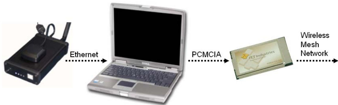
Figure 5.3: Network Subsystem Hardware: \mu WIP (left), Dell Latitude Laptop (center), ITT WMC6300 - mesh card (right)
