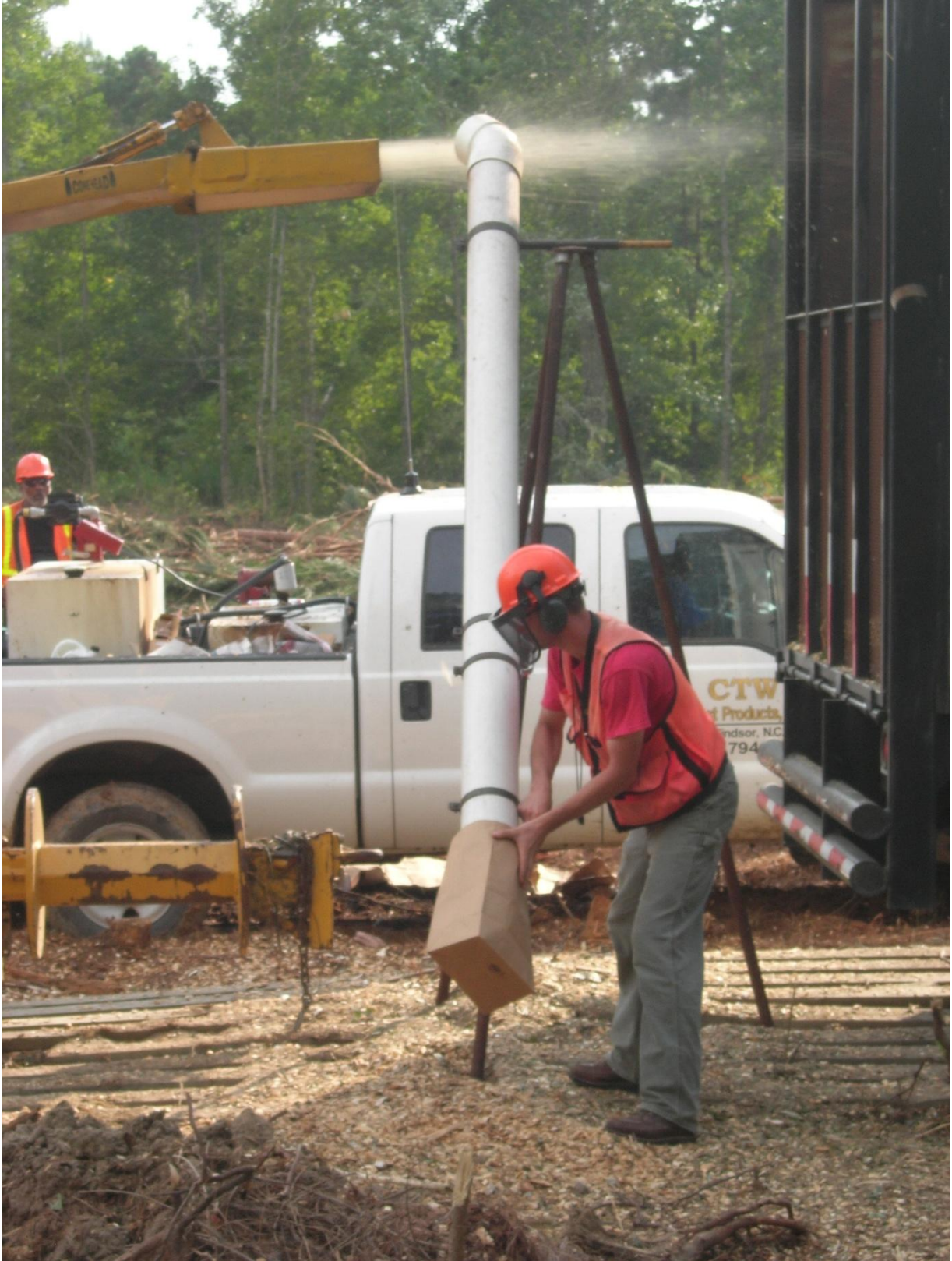
Figure 2. This image displays the method used to collect wood chips from the chip stream without causing delays in the operation of the chipper.
