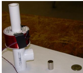
Figure 3.1. Free fall test assembly and a neodymium magnet. A quarter is shown for size comparison.
