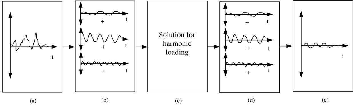
Figure 4.4 Process of Fourier transform: (a) Time history of loading, (b) Representation of time history of loading as sum of series of harmonic loads, (c) Calculation of response for each harmonic load, (d) Representation of response as sum of series of harmonic responses, (e) Summation of harmonic responses to produce time history of response (after Kramer, 1996)
