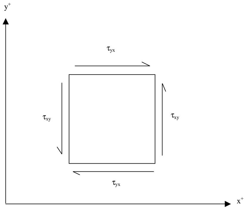
Figure 4.2 Sign convention for positive shear stresses (after FLAC, 2000)
