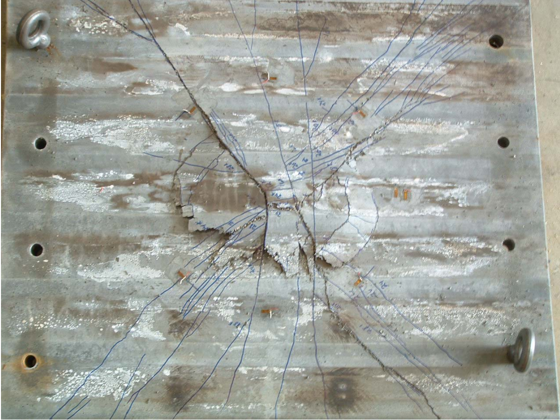
Figure B-38 – Failure Surface (2.5 in. slab – 1.5 in. plate)
