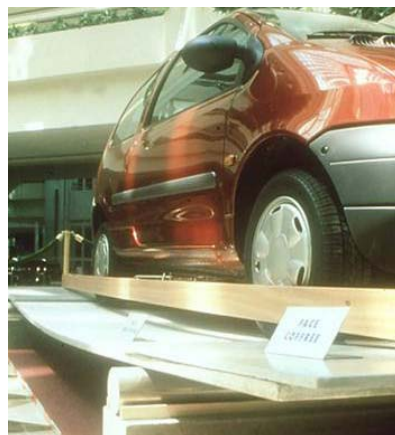
Figure 2-3 - 1 in. thick 6 ft x 10 ft slab supporting 2,000 lb car
