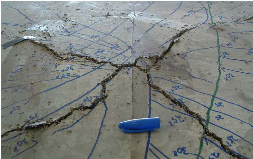
(a) Tensile face of typical slab failing in flexure
