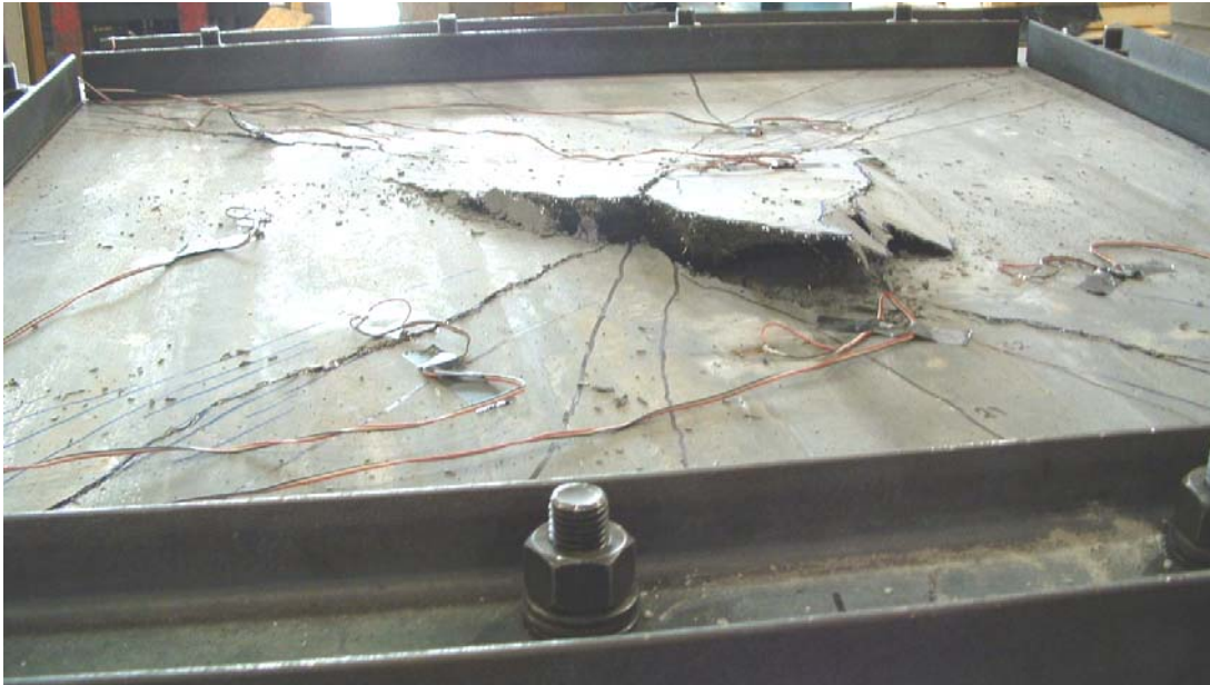
(a) Tensile face of typical slab failing in punching shear
