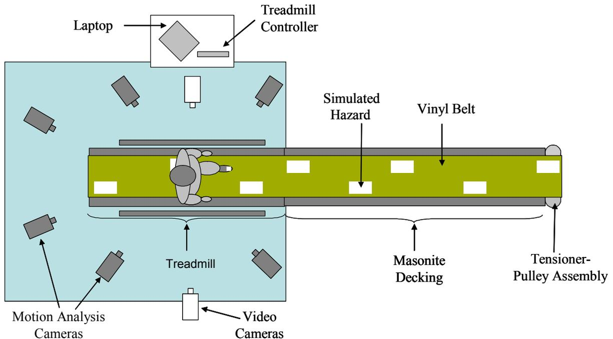
Figure 4. Test setup with modified treadmill and simulated ground hazards.
