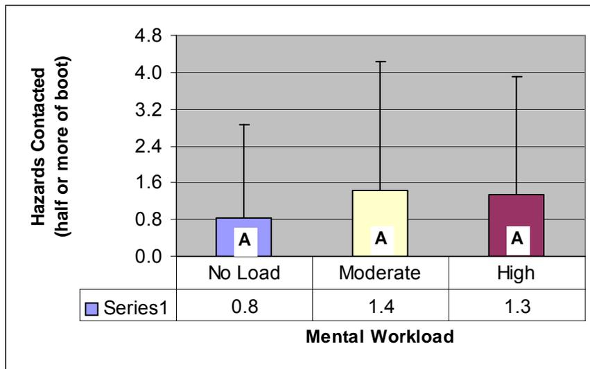
Figure 27. Mean number of hazards contacted by a minimum of one-half of either of the participant's boots at each level of mental workload.
