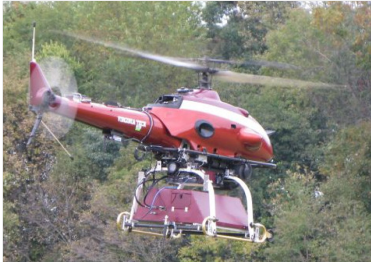
Figure 3.8: Yamaha RMAX with Radiation Detector Pod
