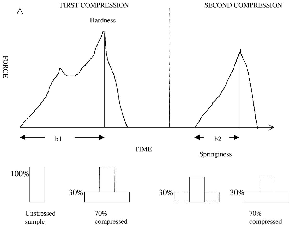
**Fig. 14:** The schematic of typical Texture Profile Analysis curves using an Instron Universal Testing Machine
