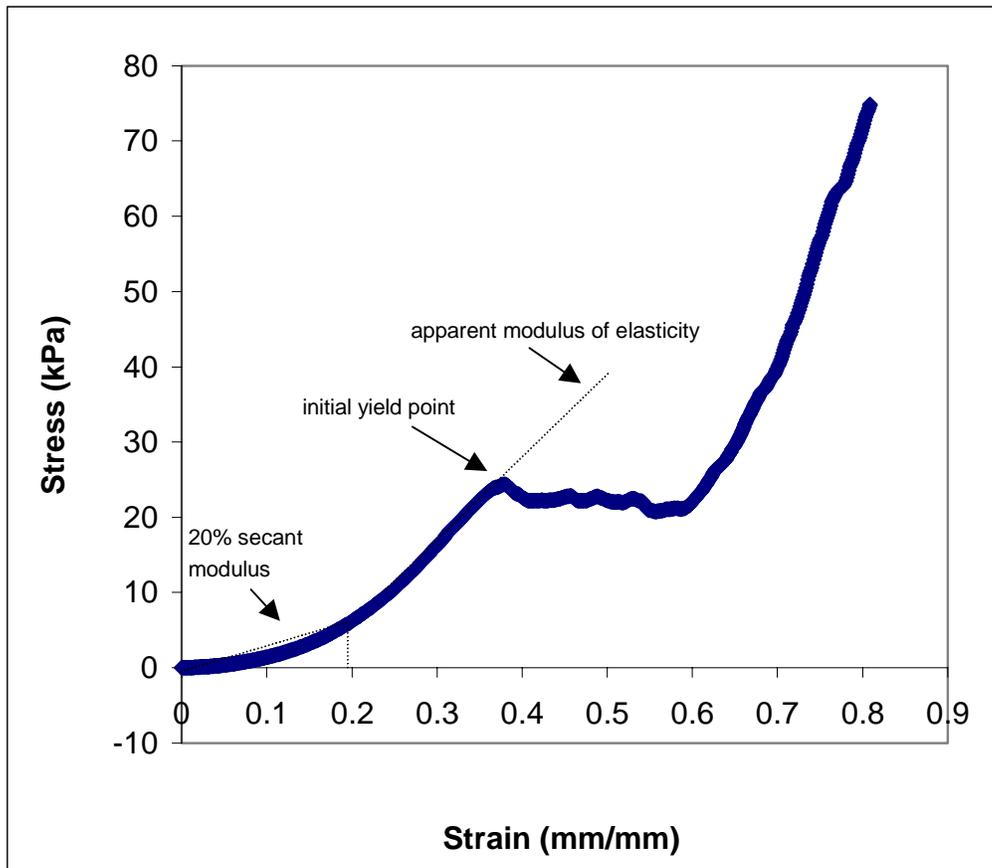
**Fig. 22: The stress-strain curve of restructured scallops with 1% alginate set at 5 °C for 2 hr derived from compression test using MTS Universal Testing Machine at the crosshead speed of 100 mm/min.**
