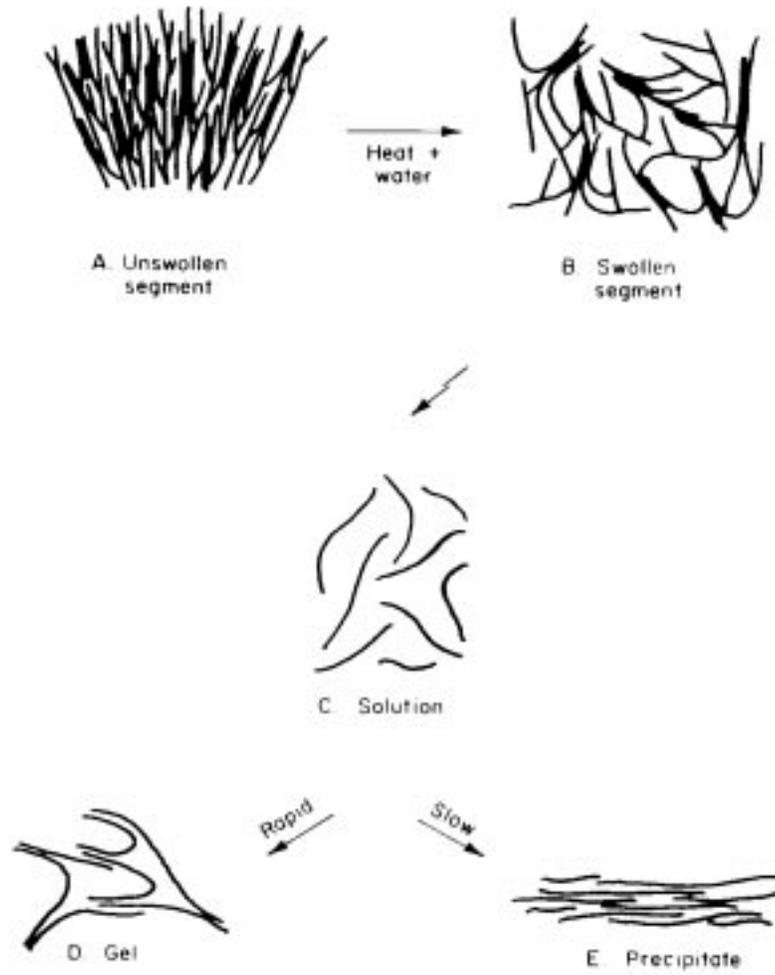
**Fig. 6: The Gel Formation of Starch (Glicksman, 1969)**
