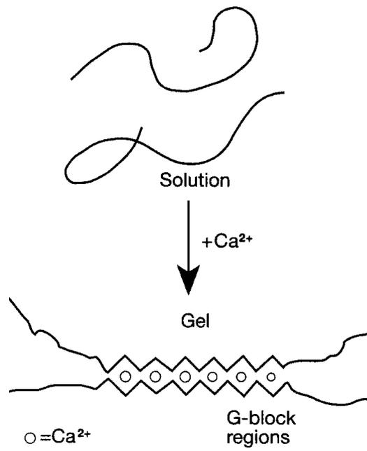
**Fig. 10: The “egg-box” structure (Anon)**
