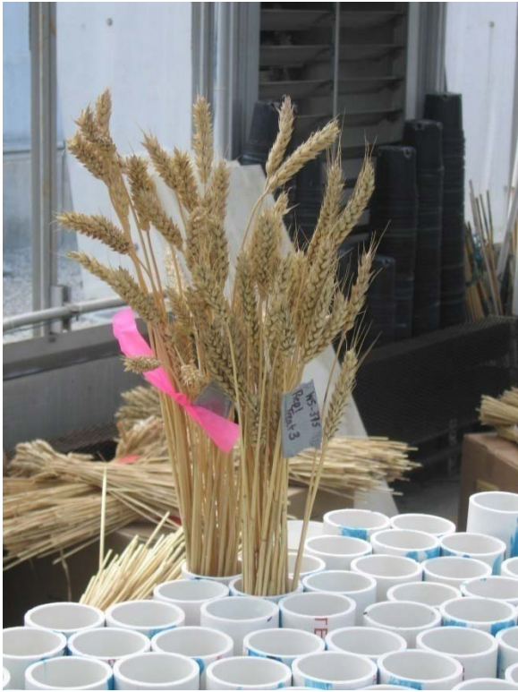
Figure 1.1. Honey-comb device used to administer simulated rainfall.
