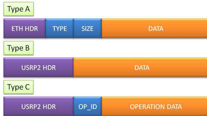
Figure 3.3: Packet formats for different channels (figure from [10])
