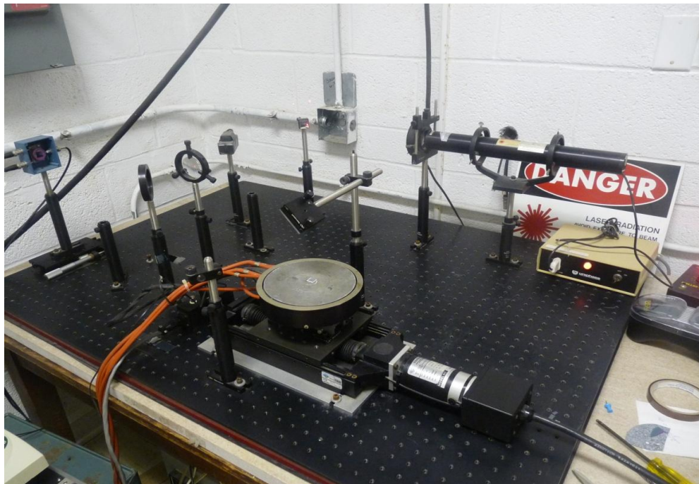
Figure 3.6. The optical setup for the curvature measurement.
