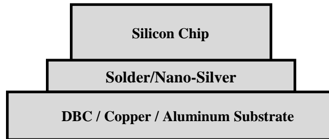
Figure 2.1. Structure of die-attachment.
