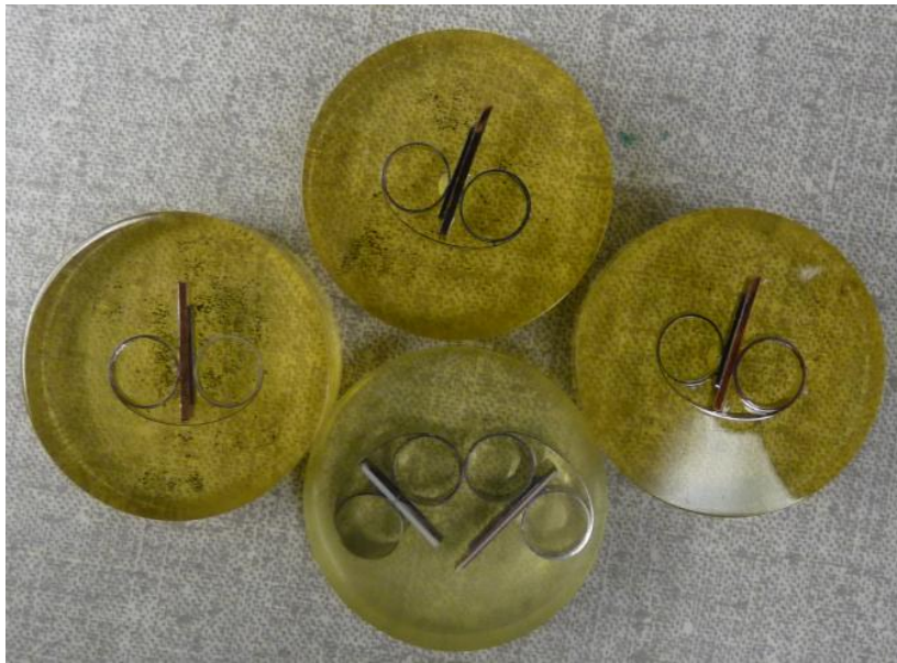
Figure 3.13. Cross-section sample in epoxy after polishing.
