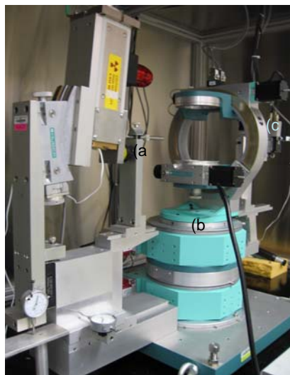
Figure 2.5 Huber picture: Picture of the Huber diffractometer with the (a) X-ray source, (b) Eulerian four-circle cradle, and (c) point detector labeled. Photograph taken by author.
