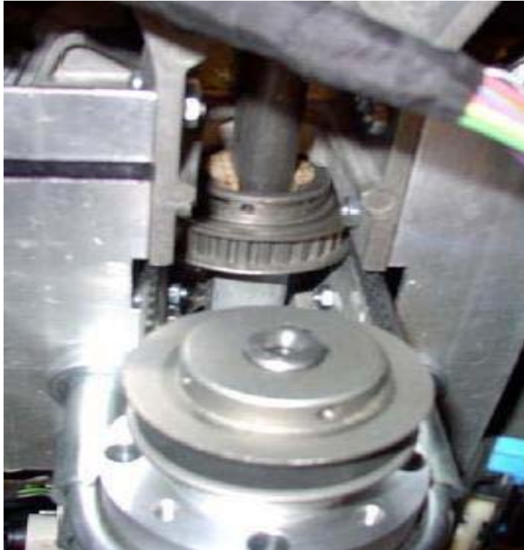
Figure 28: The final steer-by-wire belt drive system driven by the QuickSilver smart motor and a belt drive system
