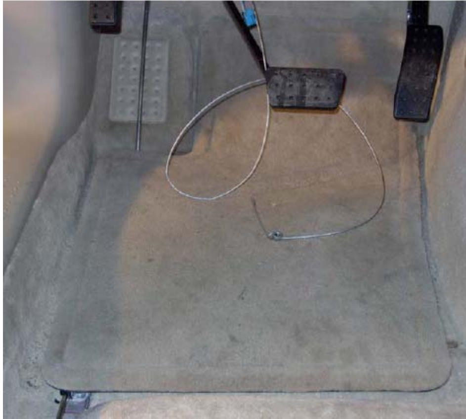
Figure 6: The final HSAVT brake-by-wire system
