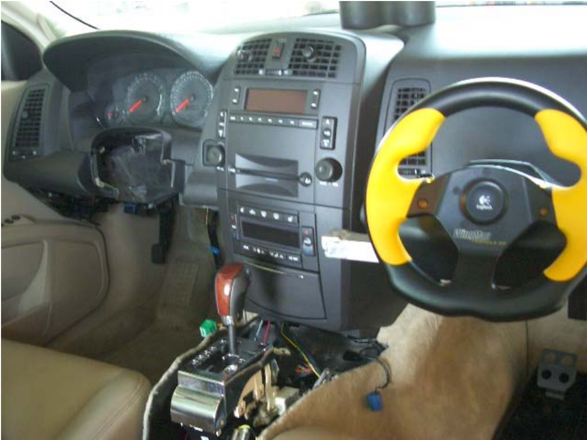
Figure 7: The Logitech Wingman Formula GP controller mounted inside of the SRX
