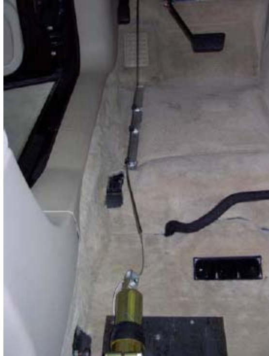
Figure 5: The HSAVT brake-by-wire solution
