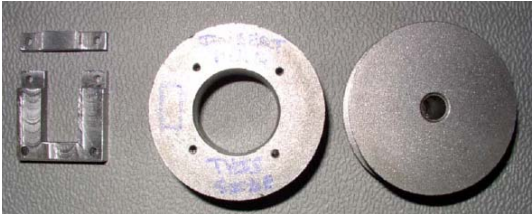
Figure 19: The adapter, pulley 2, and pulley 1
