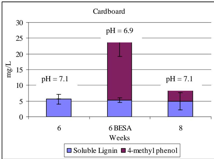
**Figure II - 10:** Soluble lignin and 4-methyl phenol accumulation at 6 weeks (BESA amended and un-amended) and 8 weeks (BESA un-amended) for cardboard.
