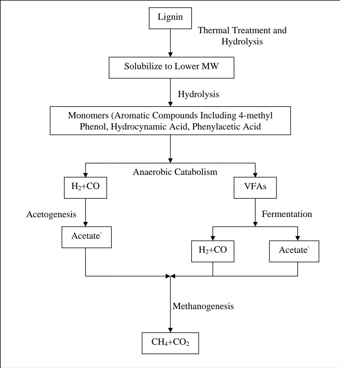
**Figure II - 7:** Anaerobic phase of carbon cycle adapted to lignin
