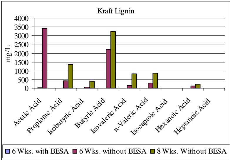
**Figure II - 13:** Volatile fatty acids accumulation at 6 weeks (BESA amended and un-amended) and 8 weeks (BESA un-amended) for Kraft lignin.
