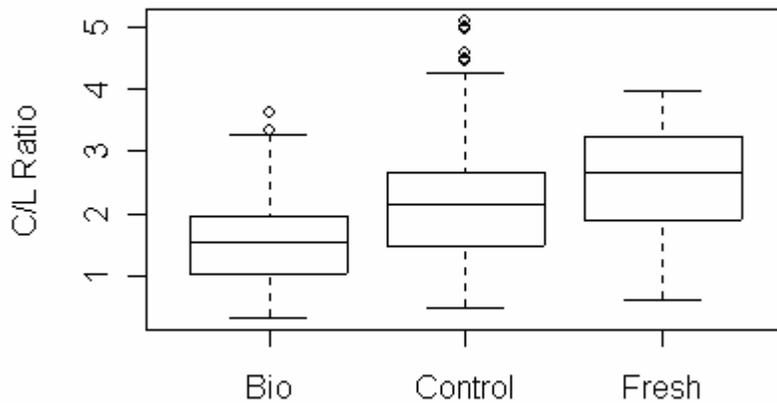
**Figure III - 1:** Box plot of the C/L Ratio for different types of MSW
