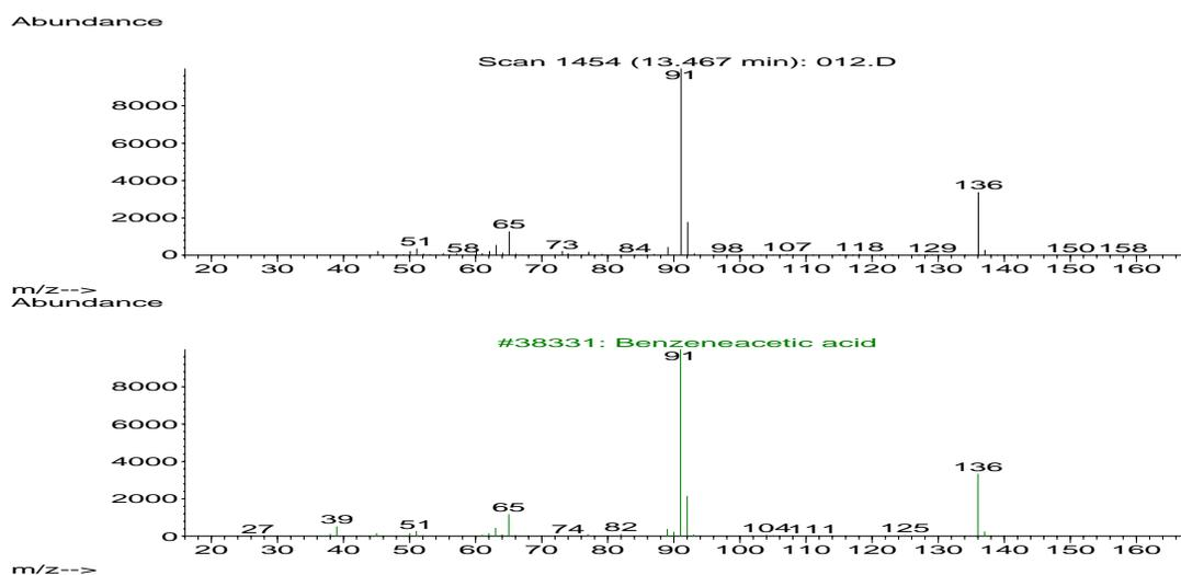
**Figure II - 9:** Ion distribution and structure for benzenoacetic acid ( $C_8H_8O_2$  2-phenylacetic acid) – lignin derived monomer.
