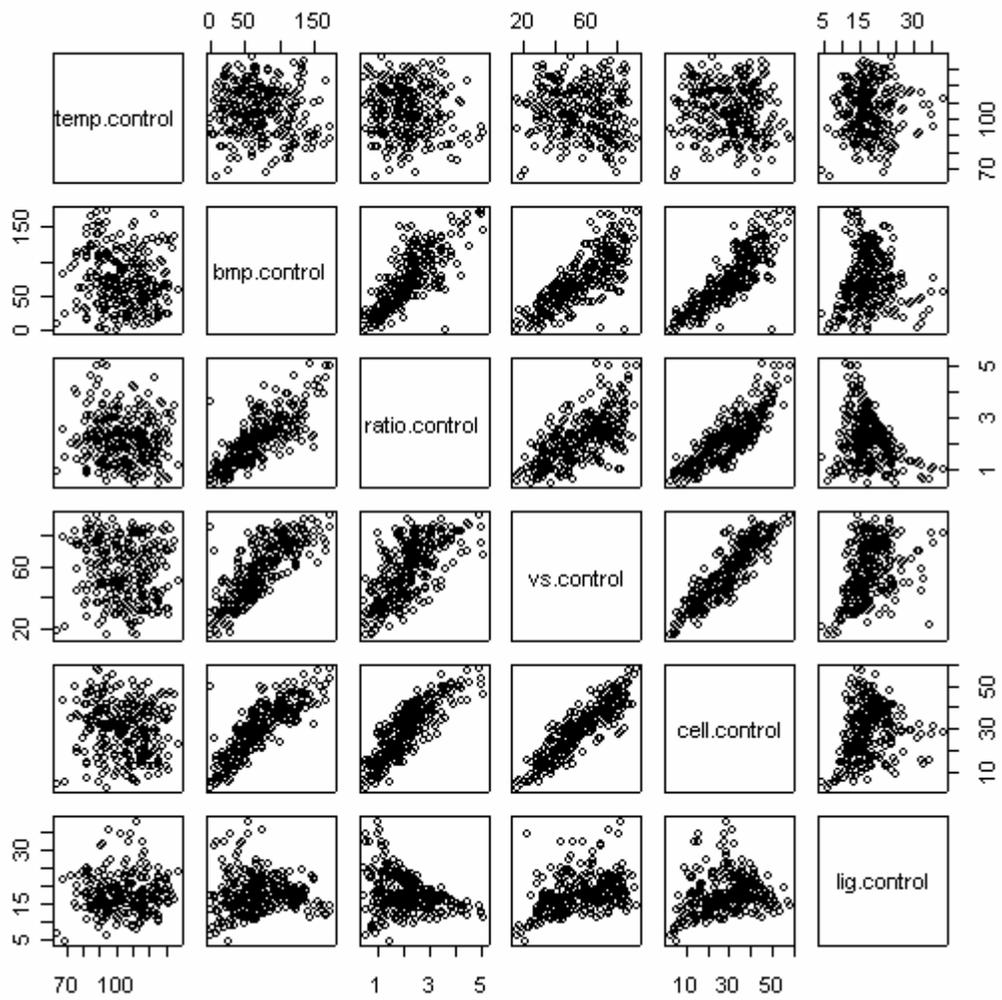
**Figure III - 10:** Scatter plot of temperature vs. stability parameters in control landfill -- temperature in °F.
