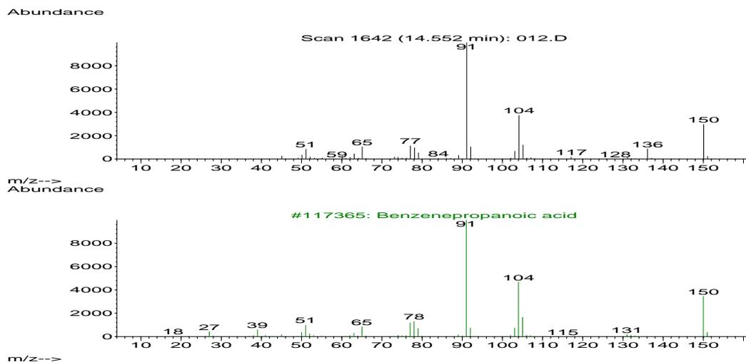
**Figure II - 8:** Ion distribution and structure for benzenepropanoic acid ( $C_9H_{10}O_2$  hydrocinnamic acid) – lignin derived monomer.
