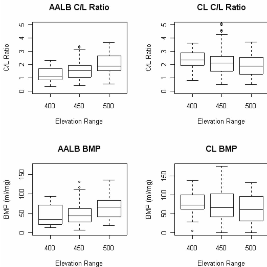
**Figure III - 5:** Box plot of the C/L Ratio and BMP over the different elevations in the landfill
