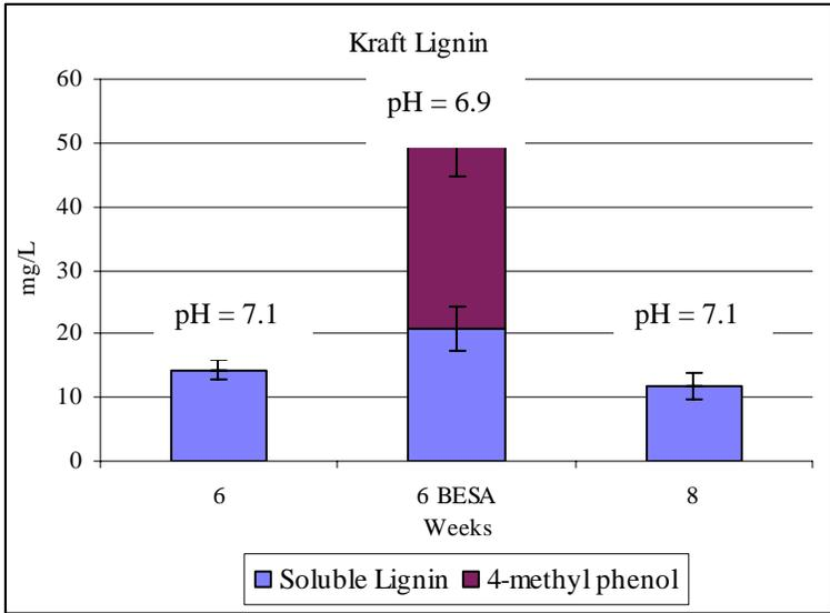
**Figure II - 12:** Soluble lignin and 4-methyl phenol accumulation at 6 weeks (BESA amended and un-amended) and 8 weeks (BESA un-amended) for Kraft lignin.
