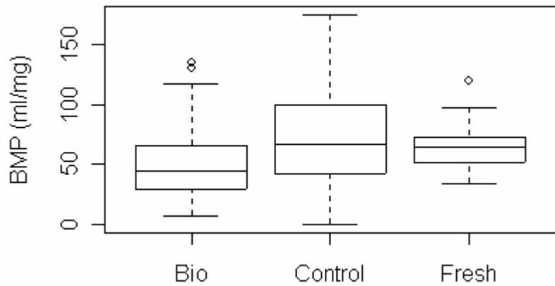
**Figure III - 2:** Box plot of the BMP of different types of MSW
