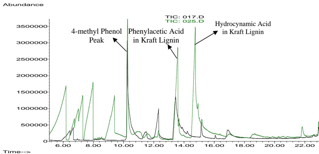
**Figure II - 15:** Chromatogram for 8 weeks Kraft lignin overlaid with 8 week blank. (Higher peaks are for Kraft lignin).
