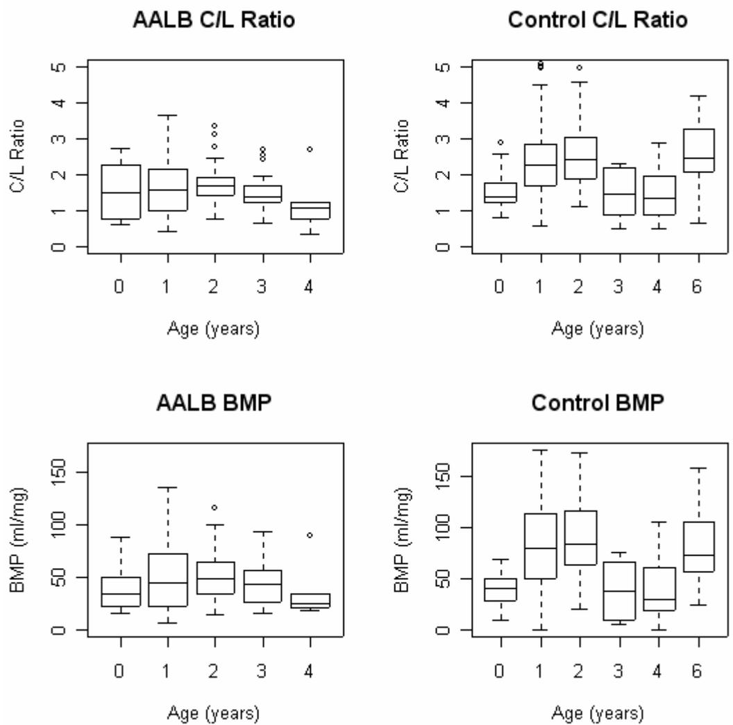
**Figure III - 4:** Box plot of the C/L Ratio and BMP over the age of the MSW (AALB and Control Landfill)
