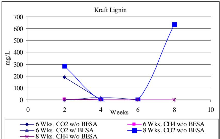
**Figure II - 14:** CO<sub>2</sub> and CH<sub>4</sub> production at 6 weeks (BESA amended and un-amended) and 8 weeks (BESA un-amended) for Kraft lignin.
