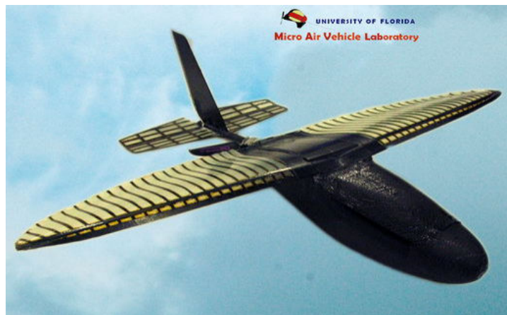
Figure 1.1 KJ Special Vision Based MAV built by University of Florida Micro Air Vehicle Laboratory (MAV Lab. University of Florida, 2007)
