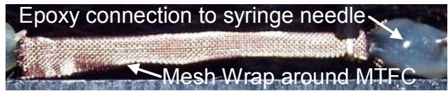
Figure 4.11 Copper mesh wrap on the cathode side as conduction layer.
