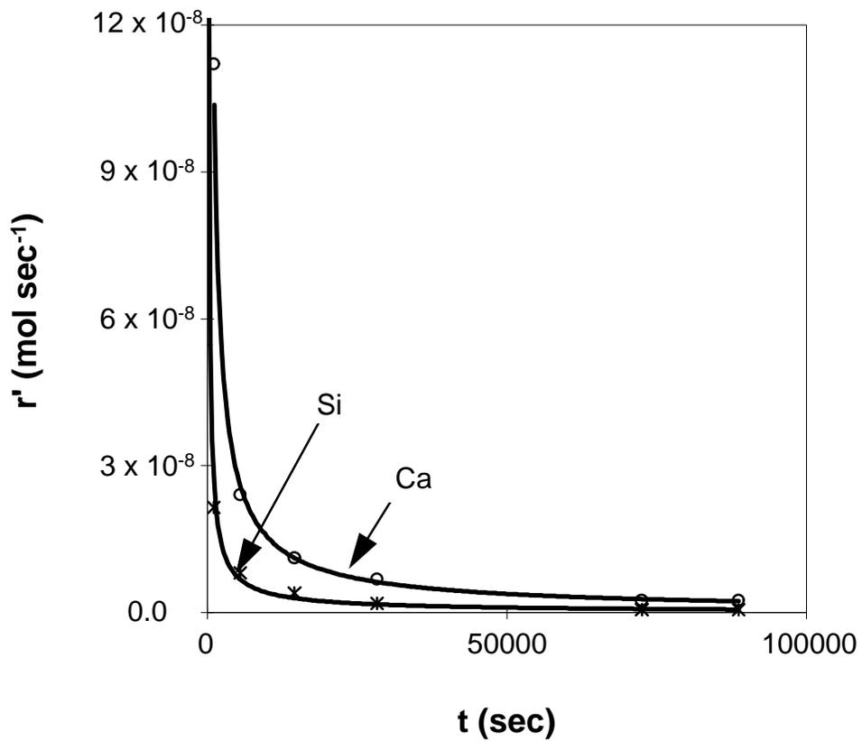
FIG. 5. Apparent release rate curves for Ca and Si from wollastonite over time for run R. These curves are typical of the release rate curves for all the experiments.
