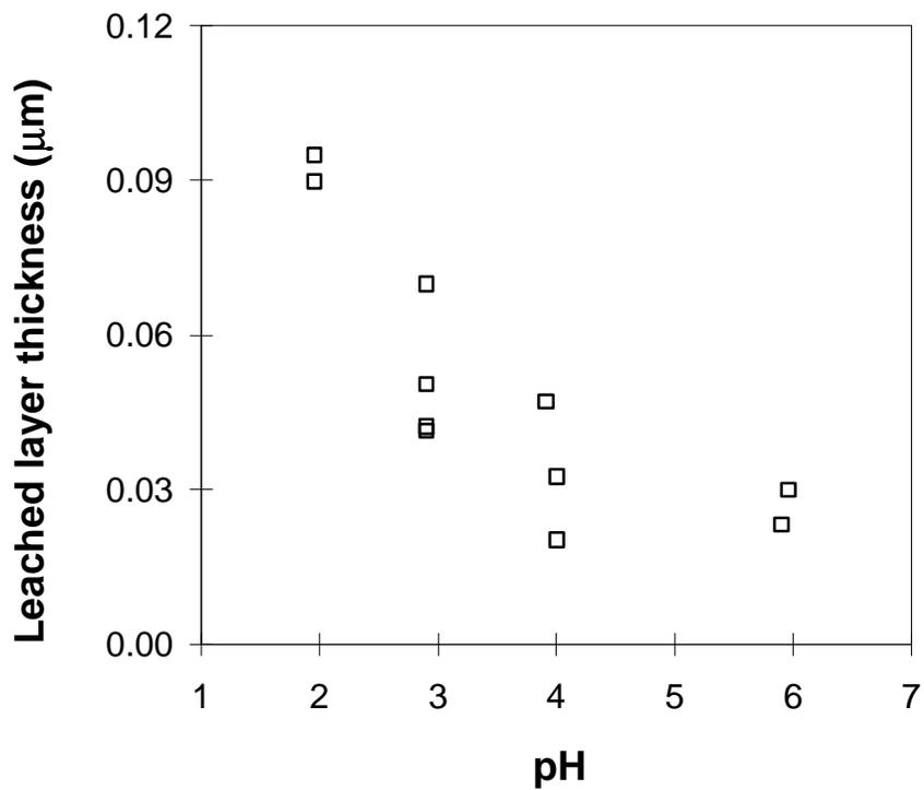
FIG. 9. Calculated leached layer thickness, using the molar volume of wollastonite, versus pH. Although there is scatter in the data due to the narrow range of the y axis, the trend shows a greater thickness of the leached layer at lower pH.
