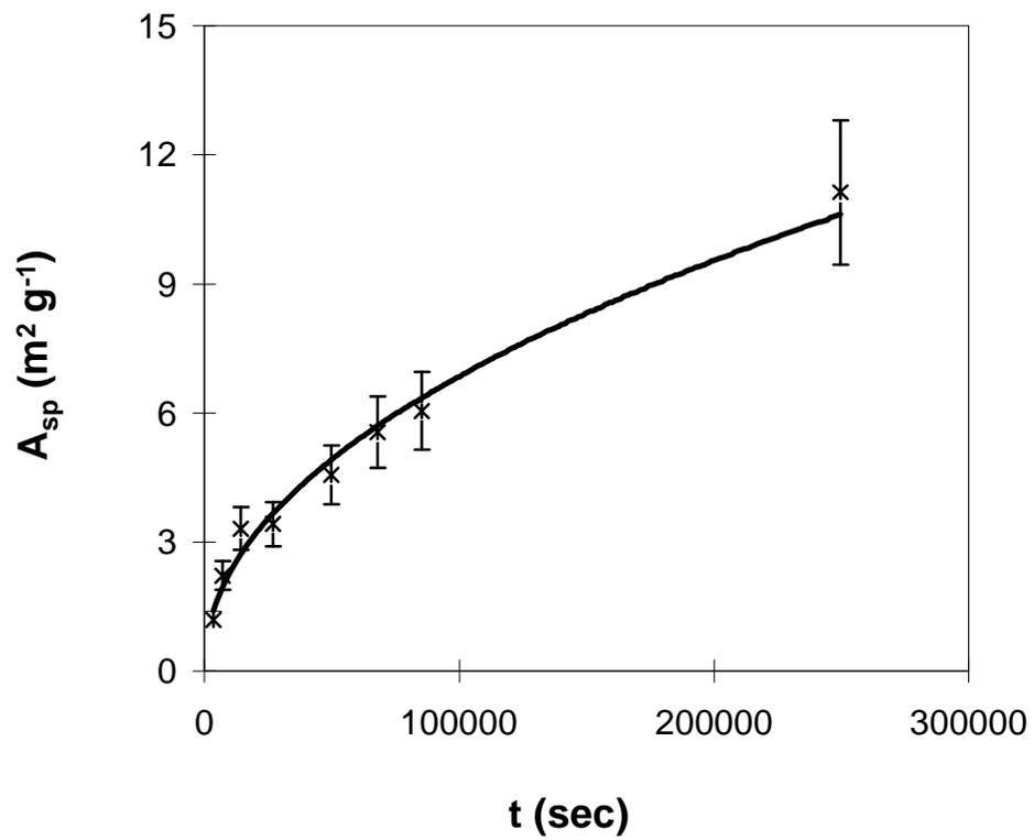
FIG. 8. The results of a series of experiments showing the evolution of BET surface area over time for wollastonite at pH 3.
