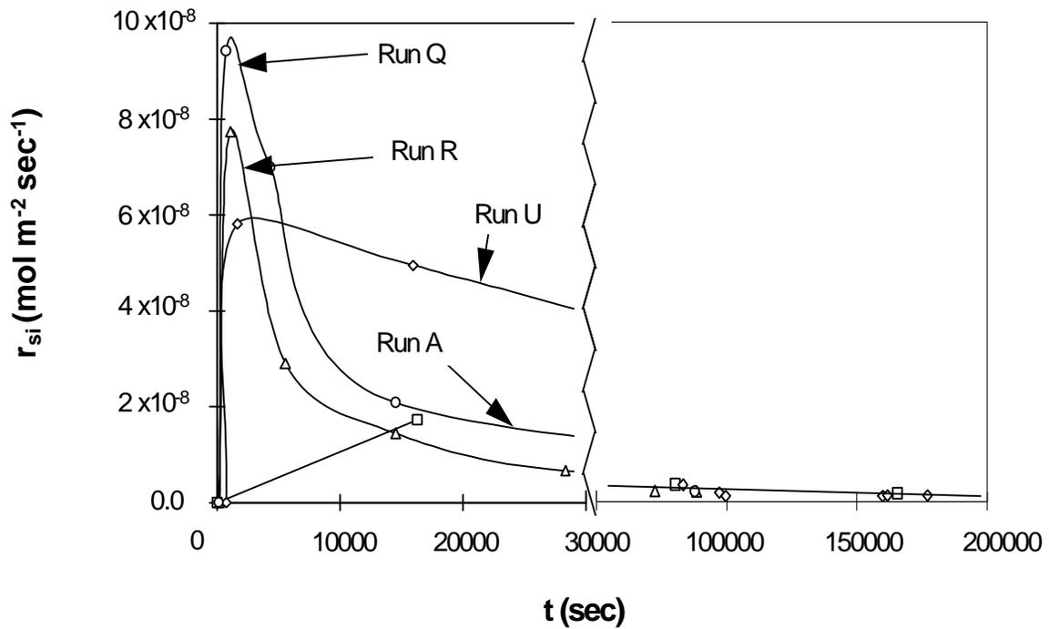
FIG. 6. Comparison of Si release rates for specified runs at pH 2.0. (See Table 1 for run conditions). The time scale has been broken at 30000 sec and been expanded to highlight the differences in initial rates and the similarities in final rates.
