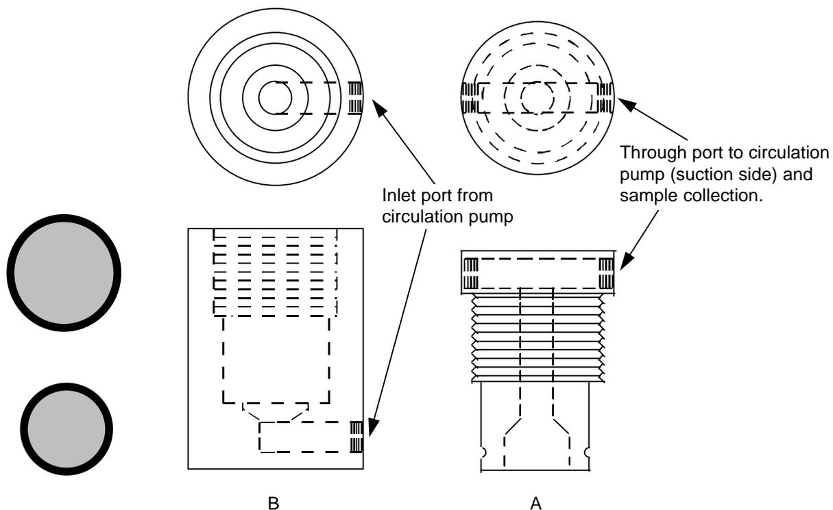
FIG. 2. Schematic representation of the Fixed bed external recycle mixed flow reactor. The material is placed into the small O-ring assembly which is inserted into the large O-ring assembly. This fixed bed of material is then inserted into "B" and held in place by the assembly of "A" into "B". A detailed version of this drawing is in Appendix C.
