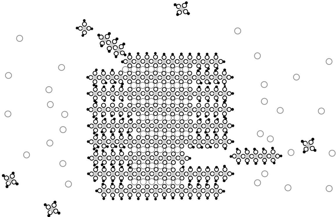
FIG. 12. Schematic representation of proposed wollastonite dissolution.  $\text{Ca}^{2+}$   $\circ$  diffuses through the Si  $\bullet$  enriched leached layer. The rate of  $\text{Ca}^{2+}$  dissolution is dependent upon
