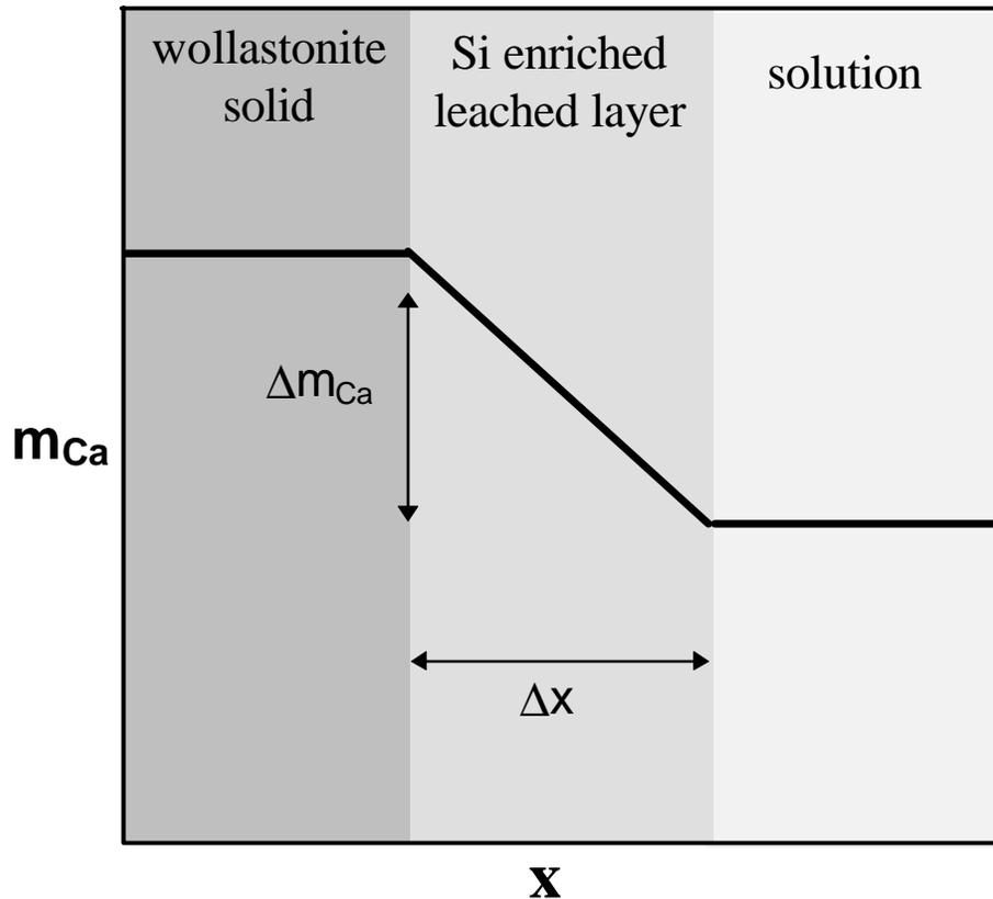
FIG. 13. Schematic representation of the wollastonite surface. Diffusion of  $\text{Ca}^{2+}$  through the Si enriched layer is dependent on the change in concentration of Ca from the solid to the solution ( $\Delta m_{\text{Ca}}$ ) and the thickness of the leached layer ( $\Delta x$ ).
