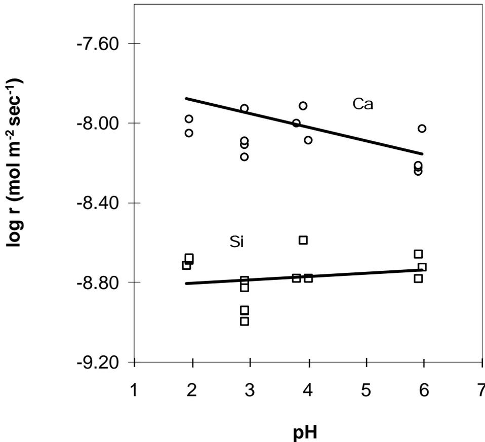
FIG. 4. Comparison of Si and Ca release rates from wollastonite for runs of 25 hour duration, from pH 2 to pH 6. The lines of best fit are  $y = 0.0168x - 8.837$ , and  $y = -0.0684x - 7.7457$  for Si and Ca, respectively.
