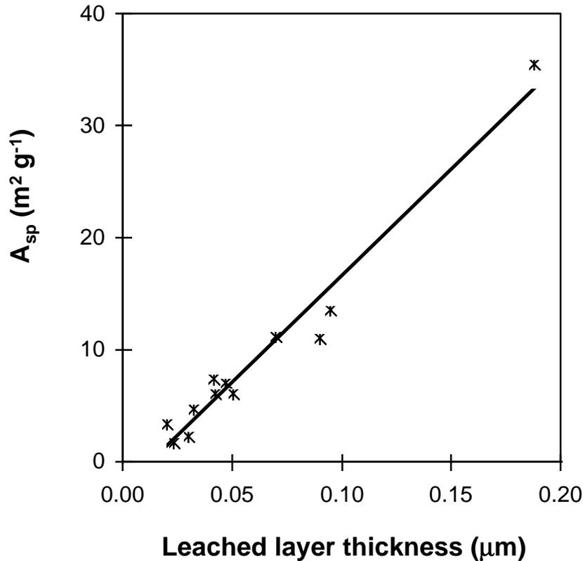
FIG. 10. Comparison of calculated leached layer thickness to measured BET surface area of wollastonite. The plot suggests that the increase in the measured surface area can be attributed to the surface area in the pore spaces of the dehydrated leached layer.
