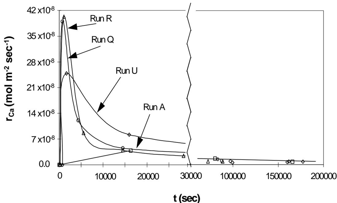
FIG. 7. Comparison of Ca release rates for specified runs at pH 2.0. (See Table 1 for run conditions). The time scale has been broken at 30000 sec and been expanded to highlight the differences in initial rates and the similarities in final rates.
