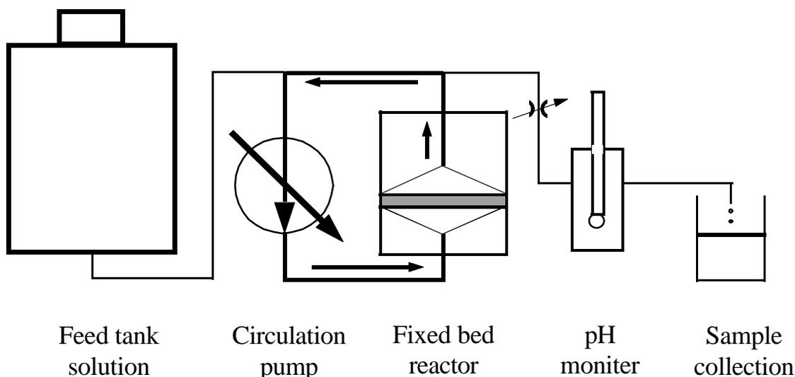
FIG. 3. Schematic diagram representing the experimental setup used in this study. The circulation pump supplied the pressure needed to circulate as well as feed the solution. The arrows trace the circulation loop through the material. Feed was regulated by a flow control valve placed in the line before sample collection.
