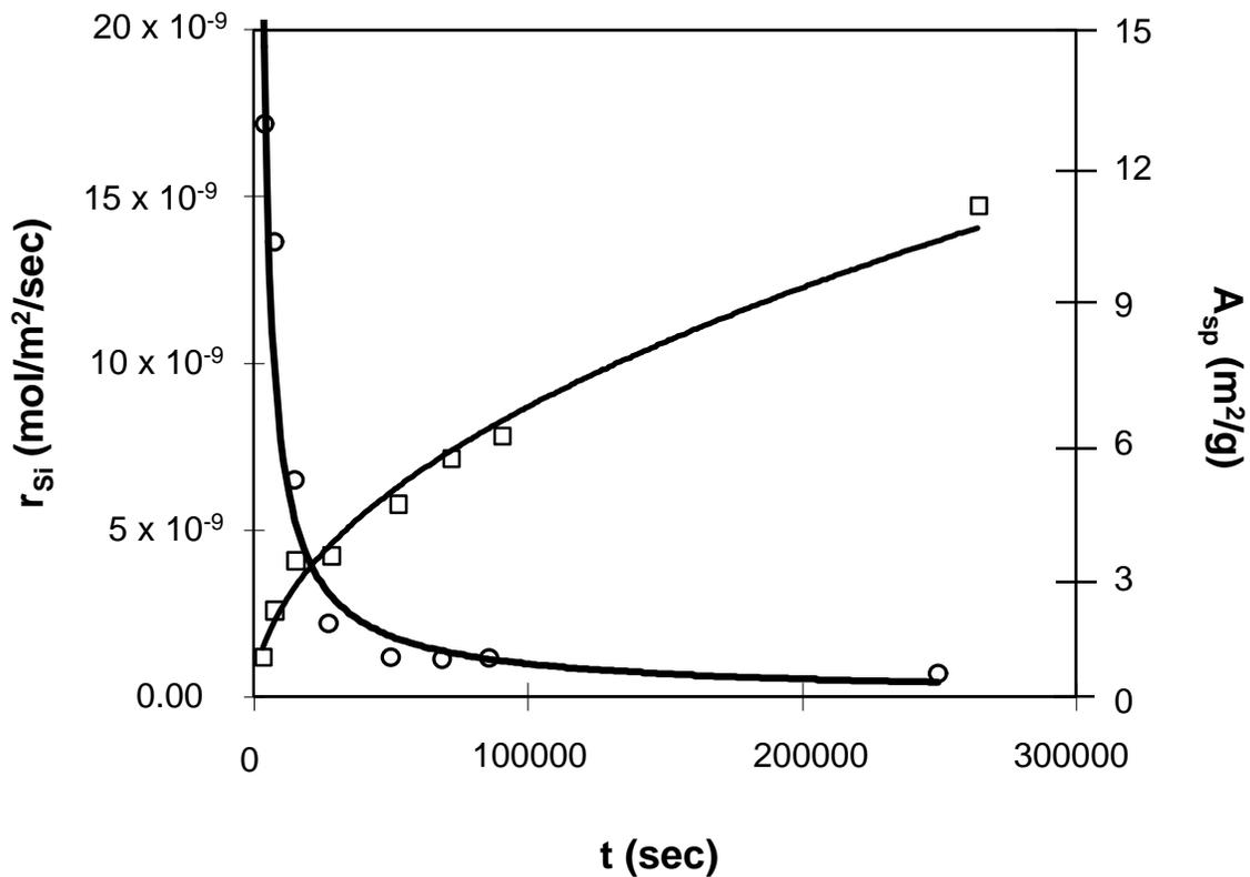
FIG. 11. Plot of Si release rate versus time for experiment Hr. This experiment showed the evolution of BET surface area by measuring  $A_{sp}$  at each time interval. It is clearly shown how the Si rate decreases with time despite increasing BET  $A_{sp}$ .
