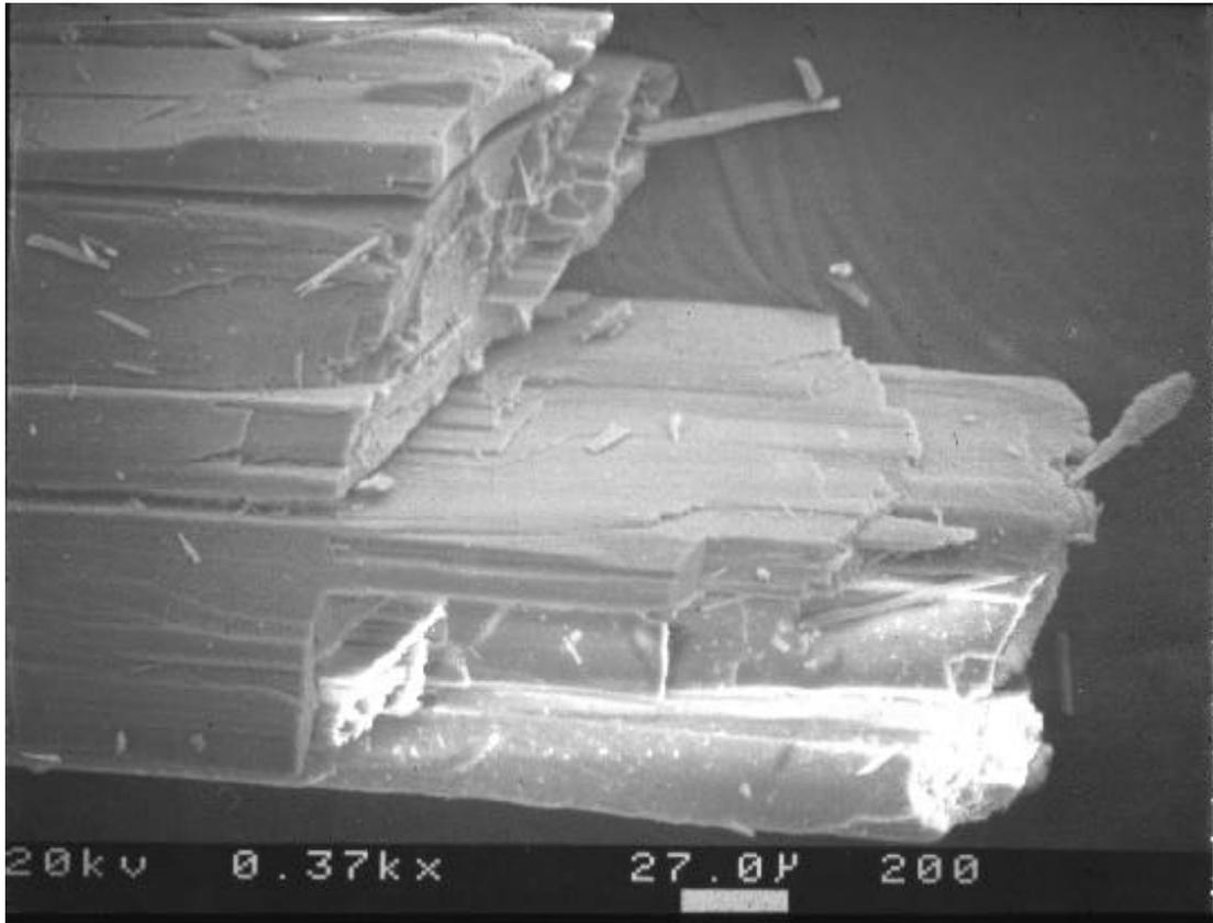
FIG. 1a. SEM photograph of unreacted wollastonite after washing and rinsing with alcohol. Though very fine particles are adhering to the surface, they do not contribute to final dissolution rates as they are quickly reacted away (See Fig. 1b).
