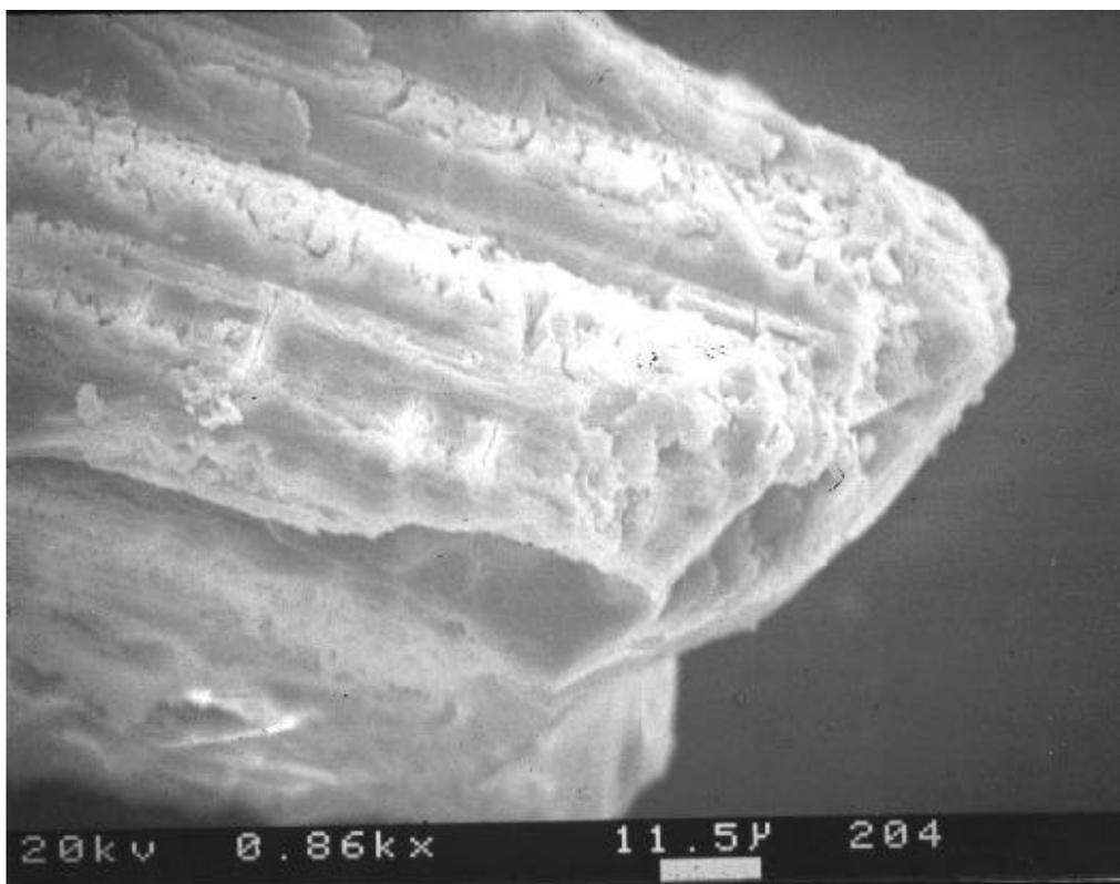
FIG. 1b. SEM photograph of wollastonite reacted for 190 hours at pH 2 in a mixed flow reactor. Though the sample has been degraded by mechanical mixing, the dehydrated Si-enriched leached layer is still visible.
