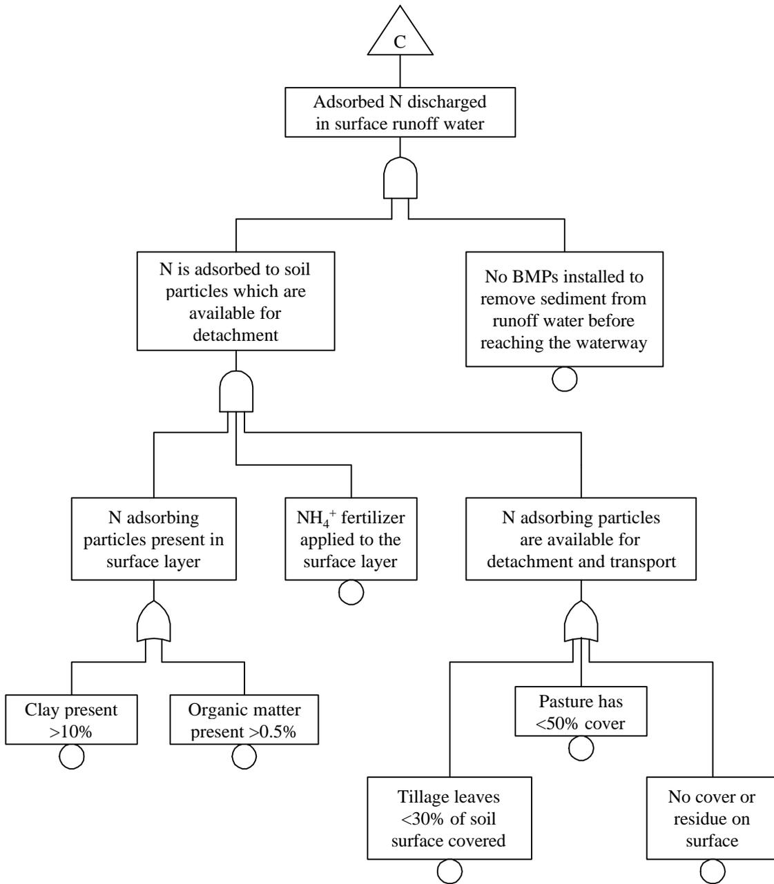
Figure 4.4: Fault tree for the discharge of nitrogen to Owl Run during a runoff event (continued)
