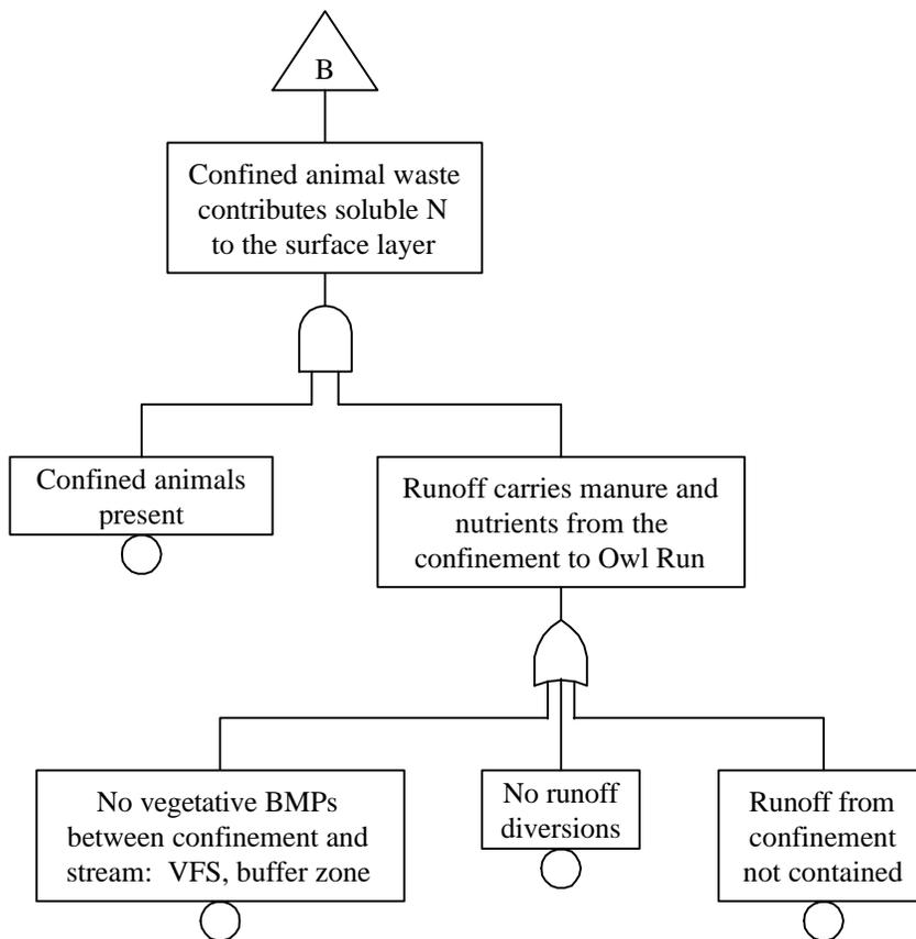
Figure 4.2: Fault tree for excessive nitrogen discharge to Owl Run (continued)
