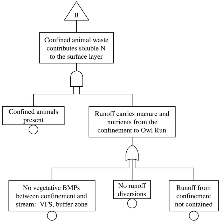
Figure 4.4: Fault tree for the discharge of nitrogen to Owl Run during a runoff event (continued)
