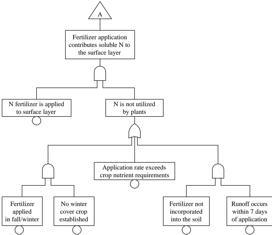
Figure 4.4: Fault tree for the discharge of nitrogen to Owl Run during a runoff event (continued)
