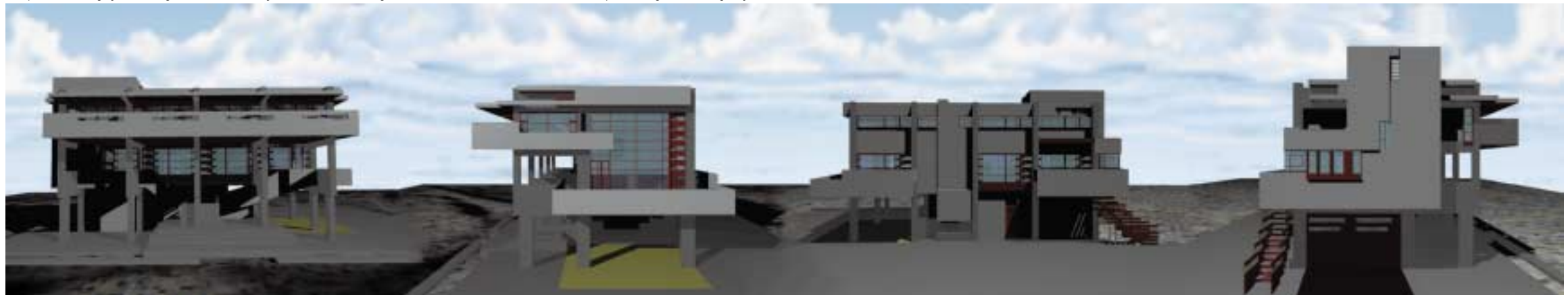
The four elevations of the Lovell Beach House as it would have appeared in 1926. These perspective elevations are computer generated using information gathered from copies of the original construction documents and archival photographs of the house taken during and shortly after construction. From left, North, West, South and East Elevations.
