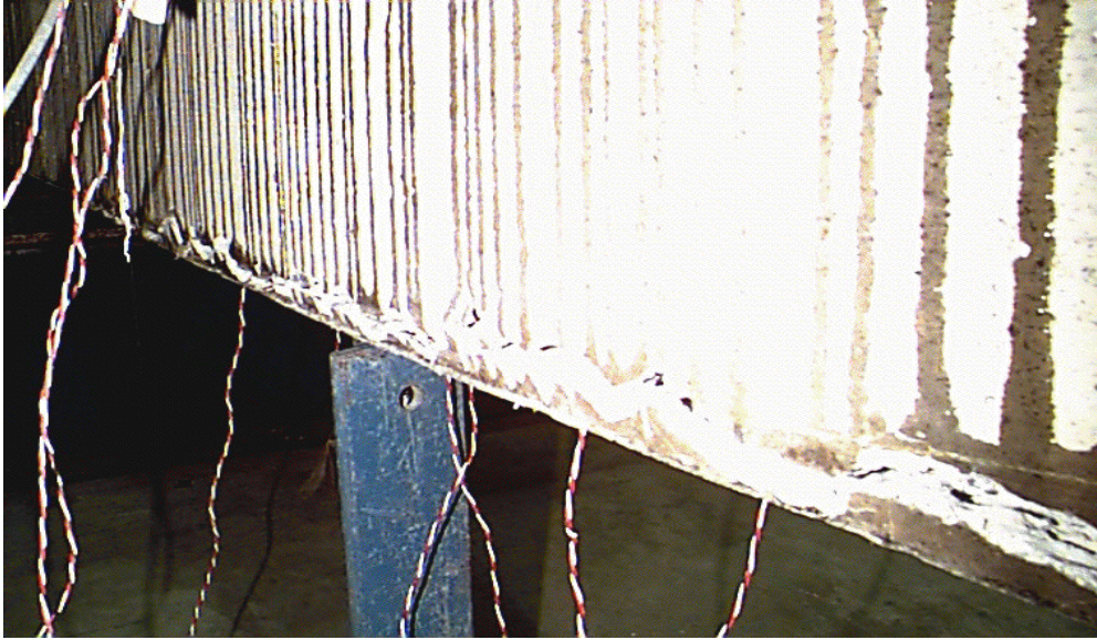
Figure 5.11: Debonding of the CFRP on Edge of Two-Layer \pm 45^\circ Composite Beam
